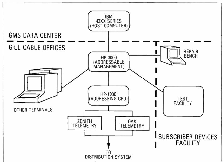
Figure 3 New computer configuration
