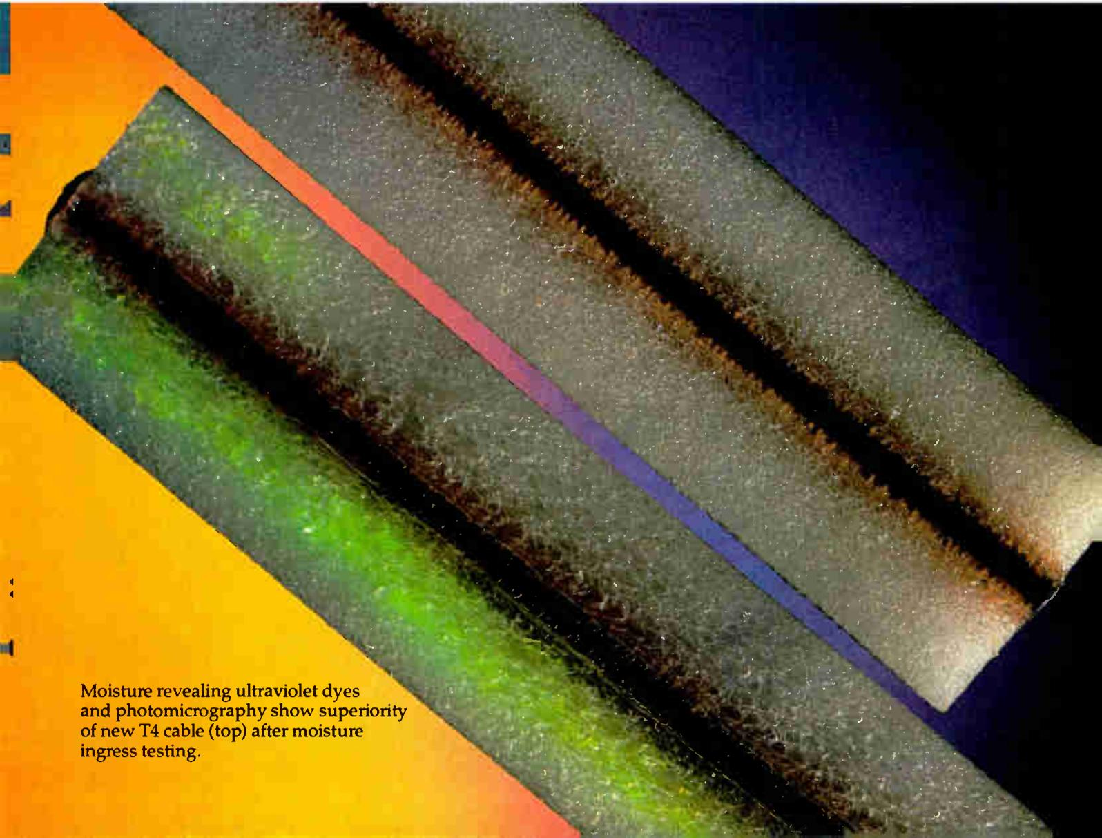
Moisture revealing ultraviolet dyes and photomicrography show superiority of new T4 cable (top) after moisture ingress testing.
