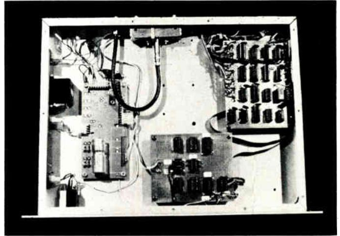
Figure 6 IEEE-488 control board added to Synchronous unit
