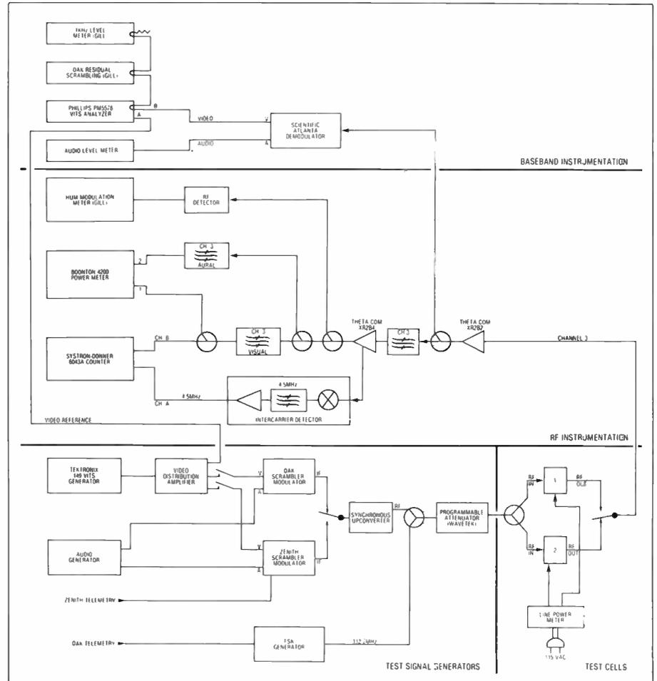
Figure 10 RF and video interconnection diagram
