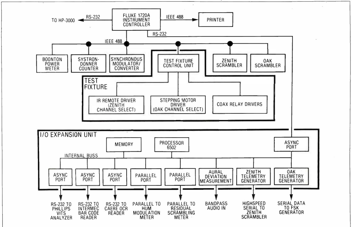
Figure 5 Control diagram-new test system
