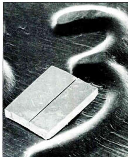
The cleaved coupled-cavity laser is a semiconductor laser cleaved into two nearly equal parts.
