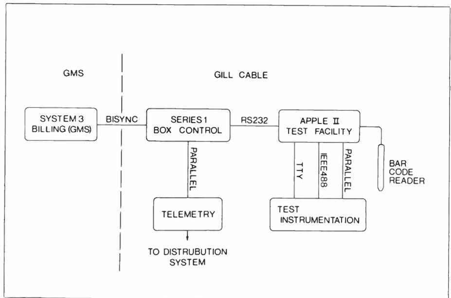
Figure 1 Original computer configuration
