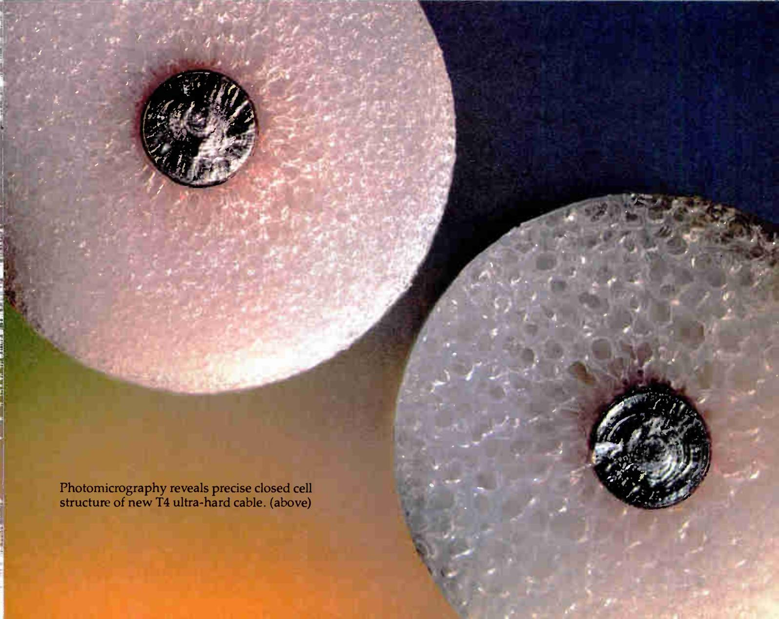
Photomicrography reveals precise closed cell structure of new T4 ultra-hard cable. (above)
