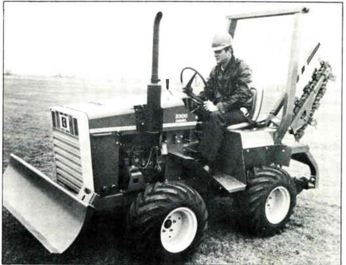
*Ditch Witch 2300 diesel trencher*
