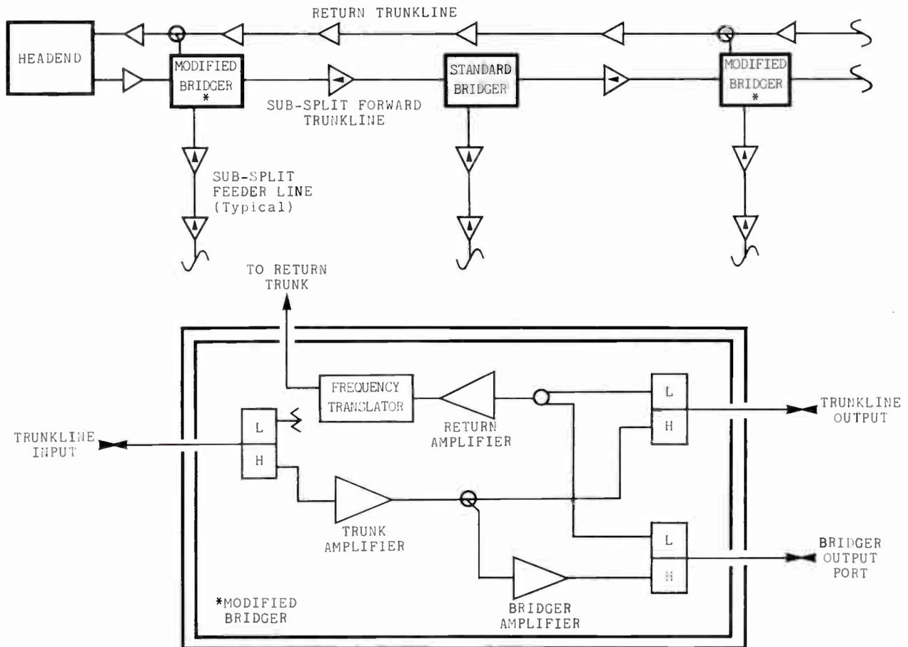
FIGURE 1 - BLOCK SEGMENT TRUNK SCHEMATIC
