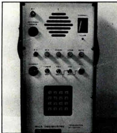
Wilk's transceiver is a portable, battery-operated unit that will function over a wide temperature range (+50 degrees C to -20 degrees C). By connecting the unit with one coaxial cable to a test point or tap, the user can communicate with similar portables anywhere on the cable system.
