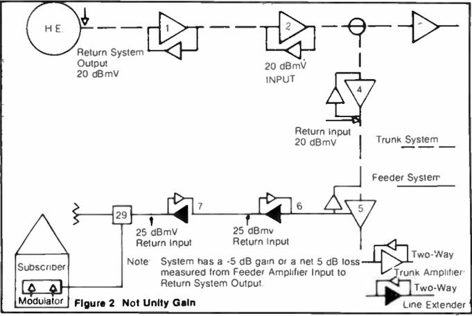
The typical system architecture applied in the United States is the forward tree structure, and the return system can be thought of as a funnel architecture. The system is segmented into two systems:
