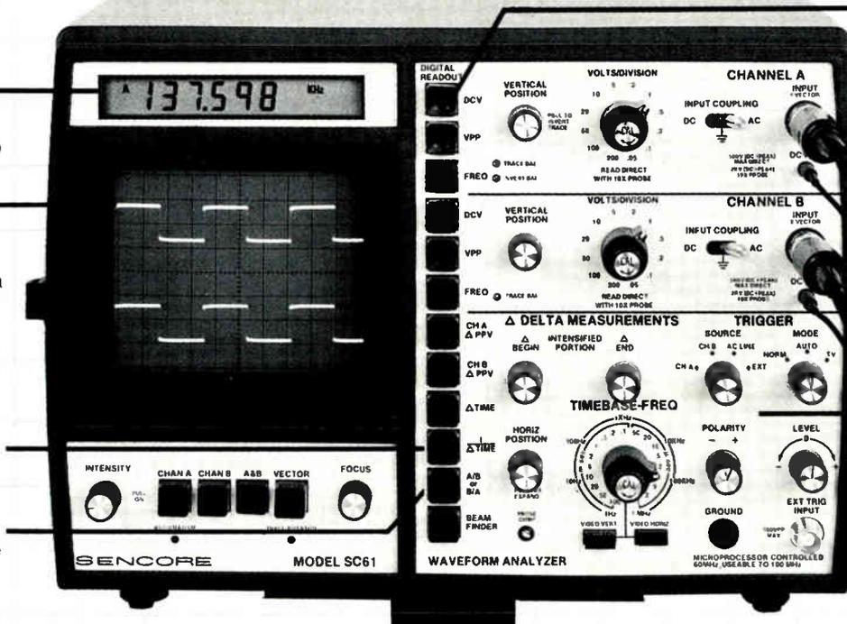
**Autotracking DCV, PPV, Freq:** Measure DCV to .5%; PPV to 2%; freq. to .001%. Just push a button for either Channel A or B.
