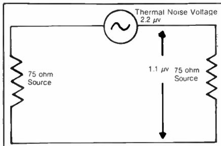
Figure 7 Thermal Noise
