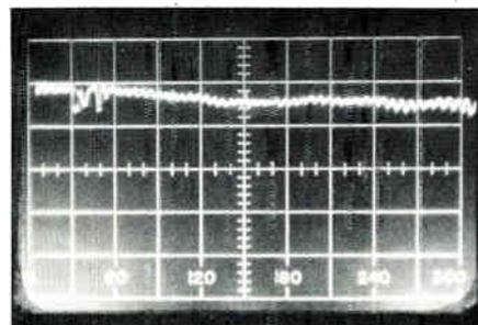
respectively. Figures 6, 7 and 8 show test results with a length of good drop cable. It is relatively easy to see what would happen to the various ripples and bumps with a length of cable which has some structural deficiencies. Figure 9 shows the test results of a length of bad cable terminated with the test resistor.
