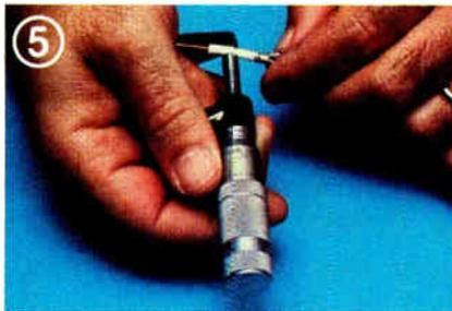
5 Measure the core in several places to make sure it is .143". On foil cables, measure over the foil to make sure it is .148". If out of tolerance, the connectors may not fit properly.
