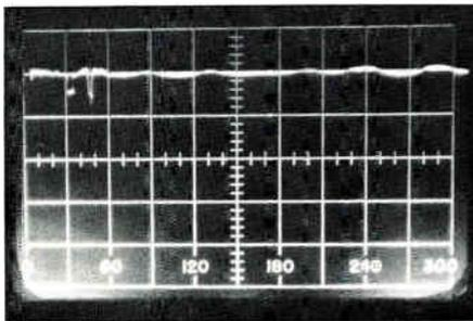
**Figure 5. Return loss of a short**
