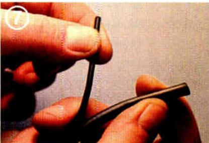
7 On messengered cable, make sure the messenger separates without tearing into the jacket and exposing the shield.
