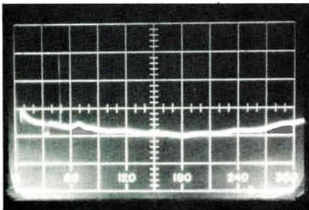
**Figure 4. Return loss of an open**
