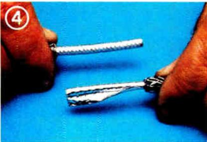
4 Now, strip off some jacket and braid, and expose the foil. If the aluminum/mylar shield peels off easily, it is not bonded. Duobond II® provides a strong bond to prevent the foil from pushing back during termination.
