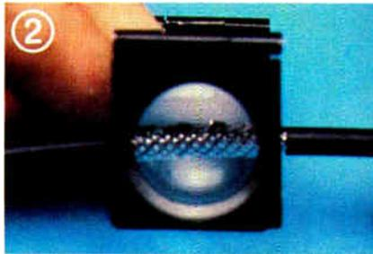
2 Carefully strip jacket off one inch of cable. If you ordered 67% braid, make sure 2/3 of the foil is covered by braid—not 1/2 or less.
