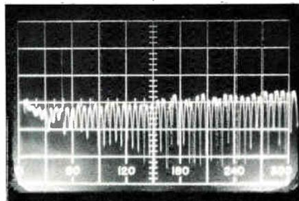
**Figure 7. Return loss of 100 ft. RG-59 shorted**
