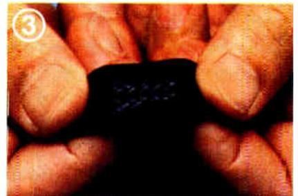
3 Check the braid impression on the underside of the removed jacket. A deep impression indicates a jacket which is too tight. This may cause difficult "F" connector installation. An extremely shallow impression indicates a jacket which is too loose.
