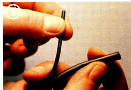
7 On messengered cable, make sure the messenger separates without tearing into the jacket and exposing the shield.
