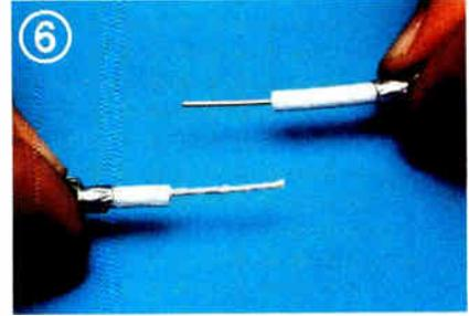
6 Remove a few inches of dielectric. If you find "fuzz" on the center conductor, intermittent contact may result. If the installer scrapes off the fuzz with a knife he runs the risk of damaging the copper cladding. Belden® cable stays smooth and clean every time.
