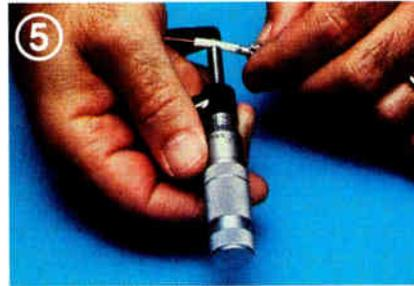
5 Measure the core in several places to make sure it is .143". On foil cables, measure over the foil to make sure it is .148". If out of tolerance, the connectors may not fit properly.
