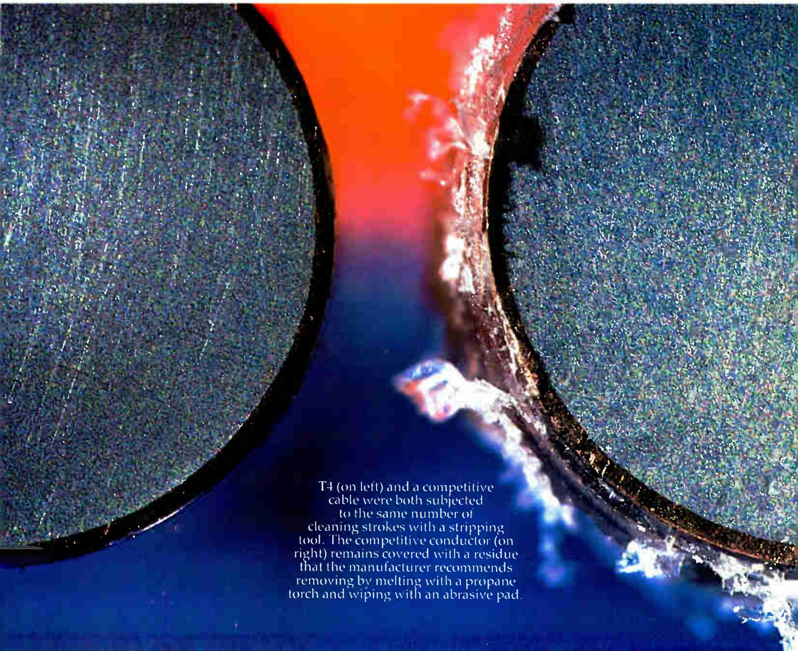
T4 (on left) and a competitive cable were both subjected to the same number of cleaning strokes with a stripping tool. The competitive conductor (on right) remains covered with a residue that the manufacturer recommends removing by melting with a propane torch and wiping with an abrasive pad.
