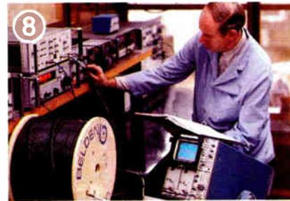
8 Is every reel of cable 100% sweep tested? All Belden® drop cable is (RG 59, 23 dB min.; RG 6, 26 dB min.). You don't have to accept anything less.
