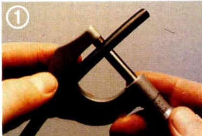
1 Measure the overall outside cable diameter with a micrometer. If it is not .242", connectors may not fit properly and performance might be affected.
