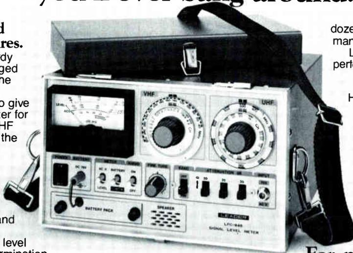
interference ratio, and image suppression ratio. For CATV, you can measure the AC power on the cable.
