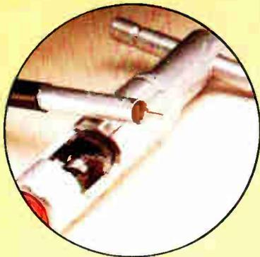
Easy coring with standard tools. Full-wall seamless aluminum tube, resistant to connectorization abuse. No objectionable non-conductive dielectric residue left on aluminum ID.
