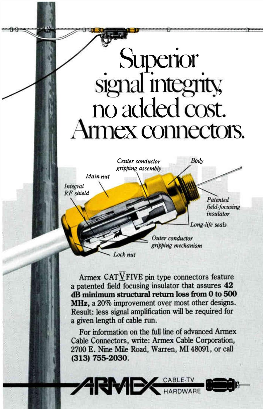
Armex CATV FIVE pin type connectors feature a patented field focusing insulator that assures **42 dB minimum structural return loss from 0 to 500 MHz**, a 20% improvement over most other designs. Result: less signal amplification will be required for a given length of cable run.
