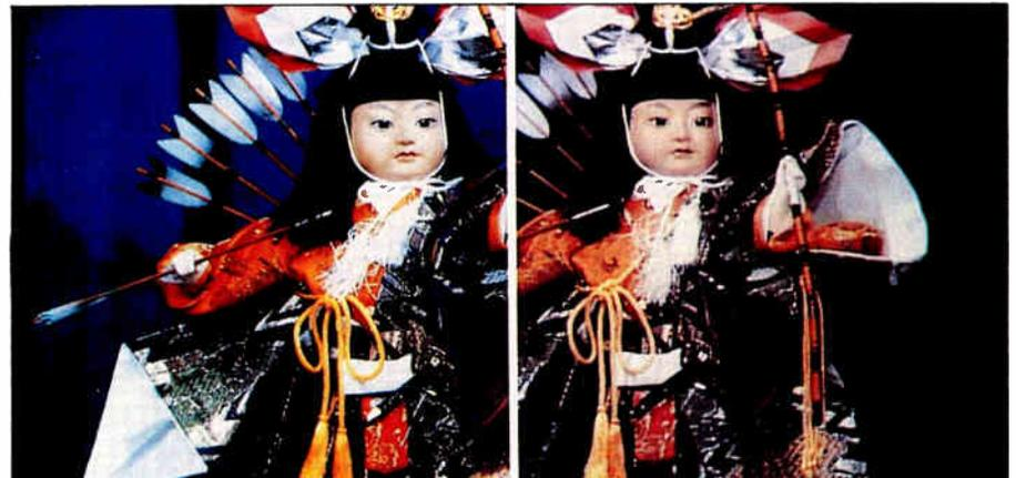
*To the left is a picture produced by Sony Corp.'s HDTV system using 1,125 lines. On right is the same picture using NTSC 525-line format.*
