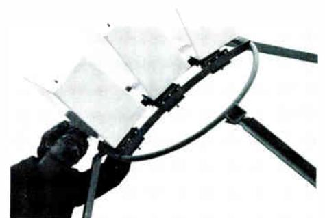
*When installed on a 5-meter antenna, isolation between beams is better than 20 dB, with a loss of about 1 dB at 4° off boresight.*
