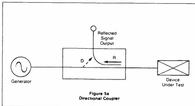
which is adequate for many applications. But if the return loss of the device under test has a return loss of 40dB, the measured return loss could vary between 34dB (both signals add) and infinity (both signals exactly cancel). Techniques such as short circuit/open circuit averaging can improve the accuracy, but generally require extra computation on a frequency-by-frequency basis.
