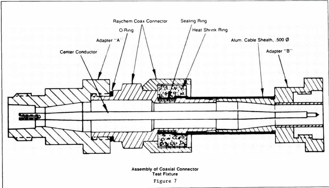
Assembly of Coaxial Connector Test Fixture
