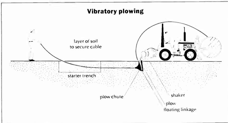
cable, since it is much faster than trenching and causes much less yard damage. It is also better than the direct plowing method because there is less chance of damaging the cable during installation.
