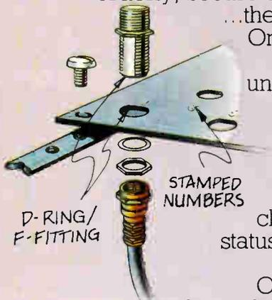
by stamped numbers on the tops of the panels. Once leads are connected, they need never be touched again—checking or changing status means handling only jumper
