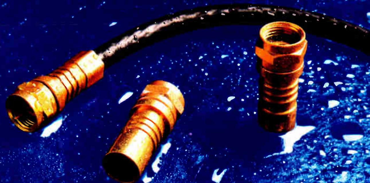
LRC Electronics introduces the DUAL SEAL "F" CONNECTOR, a premium style "F" fitting. These connectors seal to both the female post by tightening, and to the cable jacket by crimping. With the use of both rubber and silicone seals at the front and back of the connector, moisture is prevented from migrating down the braid of the cable. Keeping moisture out insures longer life to subscriber drops.
