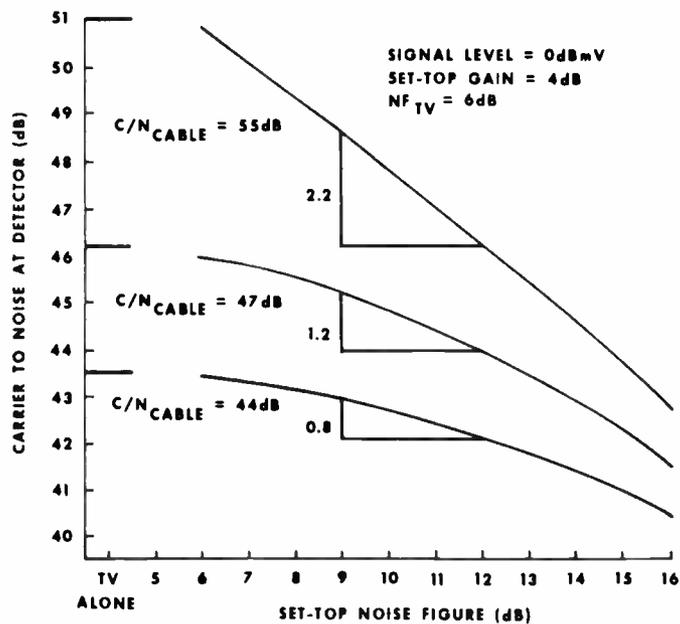
**Figure 13 Carrier to noise ratio vs. set-top noise figure**
