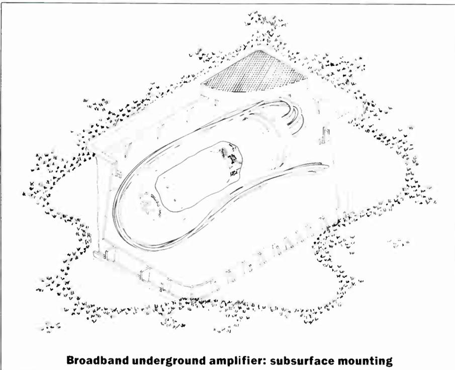
**Broadband underground amplifier: subsurface mounting**
