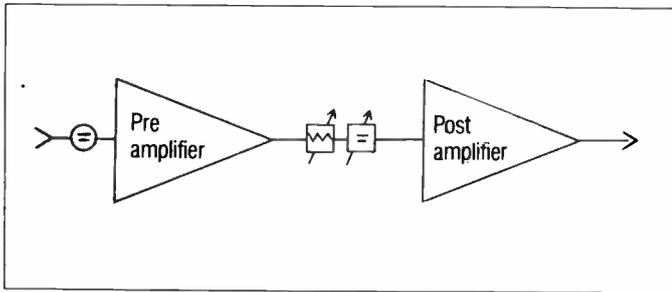
**Typical CATV amplifier block diagram**
