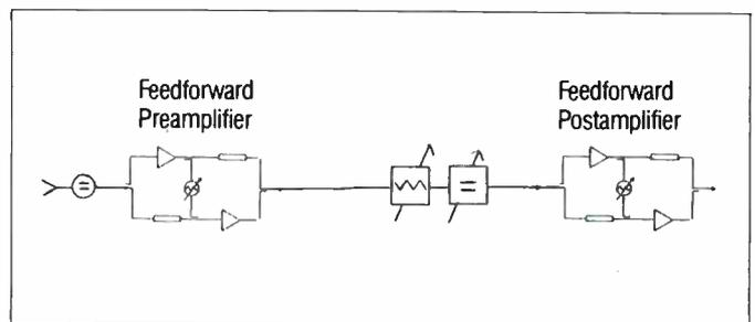
**CATV amplifier with feedforward pre- and post amplifier**
