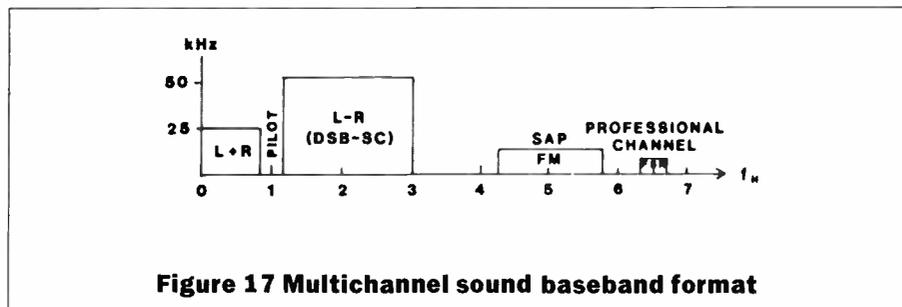
Figure 17 Multichannel sound baseband format
