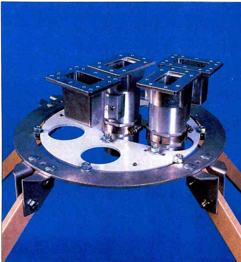
SSE performance kits™ feature individual azimuth, elevation, focal length and polarity adjustments. Fibreglass cover for protection.
