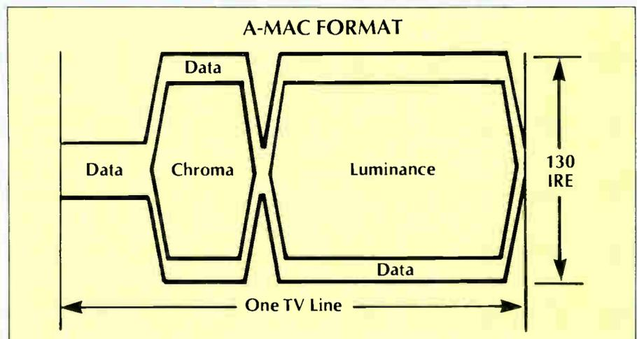
A-MAC provides a baseband frequency multiplex of the audio and data on a subcarrier.
