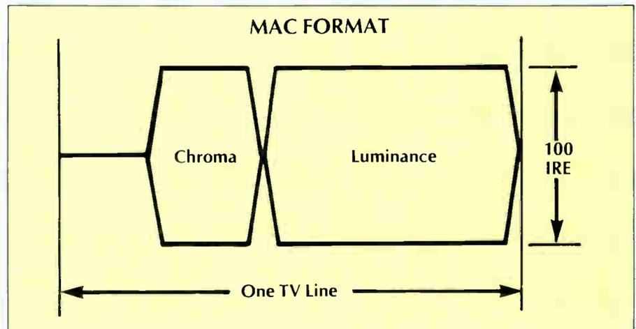
Chrominance and luminance are time compressed and transmitted in a sequential format on each TV line.
