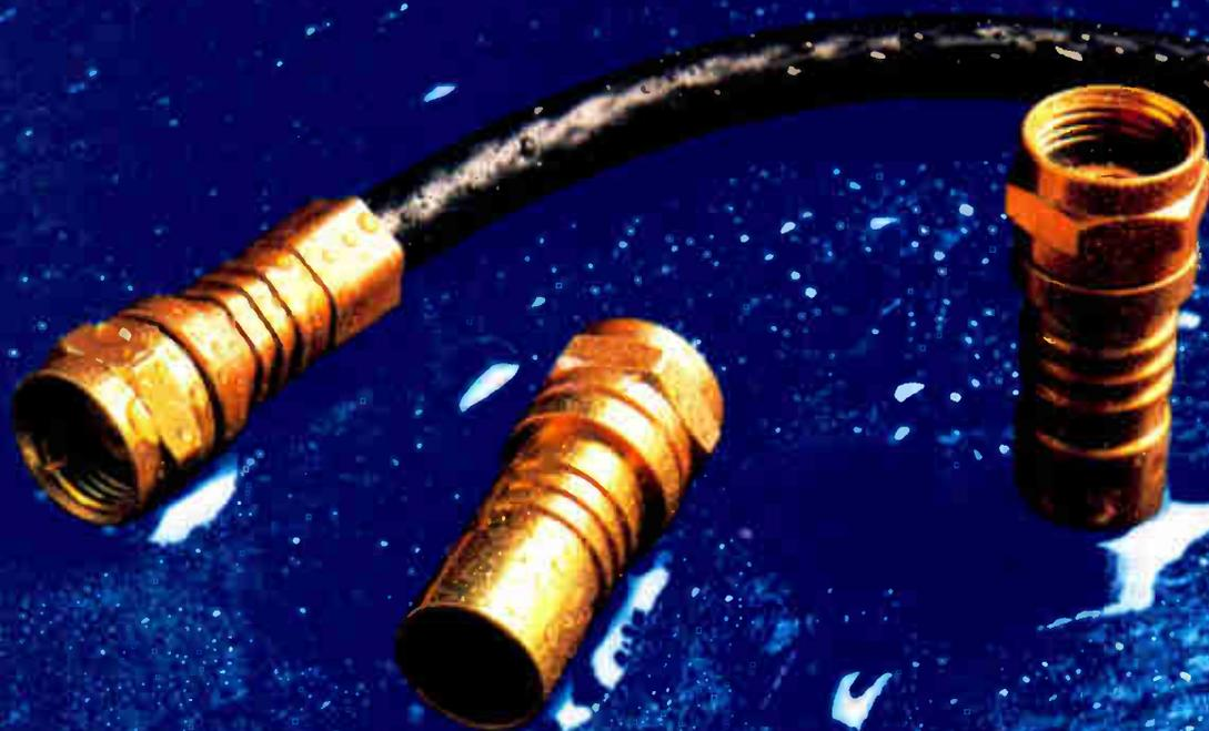
LRC Electronics introduces the DUAL SEAL "F" CONNECTOR, a premium style "F" fitting. These connectors seal to both the female post by tightening, and to the cable jacket by crimping. With the use of both rubber and silicone seals at the front and back of the connector, moisture is prevented from migrating down the braid of the cable. Keeping moisture out insures longer life to subscriber drops.
