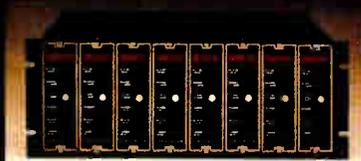
Model ZR7 rack mount with Z19 modems installed. Model ZP7 plug-in power supply also available.
