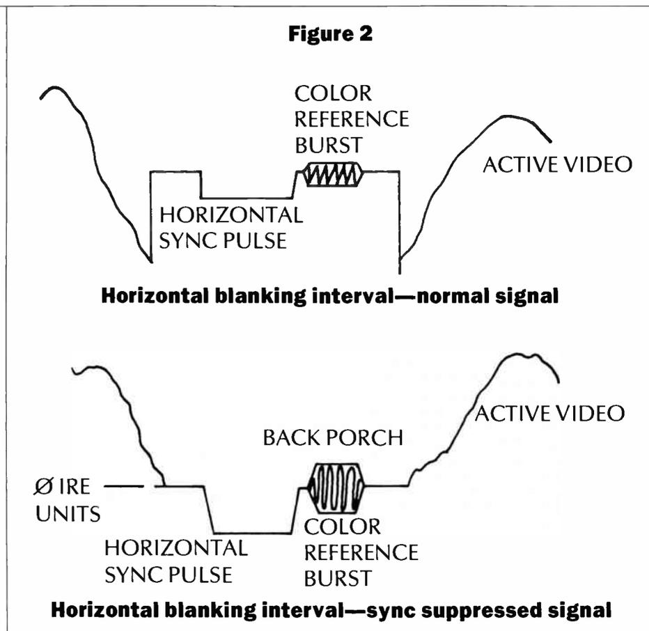
scrambling was tested, with similar results. It is important to note that the viewing parameters necessary for recovery of a sync suppressed signal are not suitable for recovery of a clear signal. Therefore, each switch between clear and scrambled signals requires reconfiguration of viewing parameters and changing of horizontal and vertical sync recovery modes.
