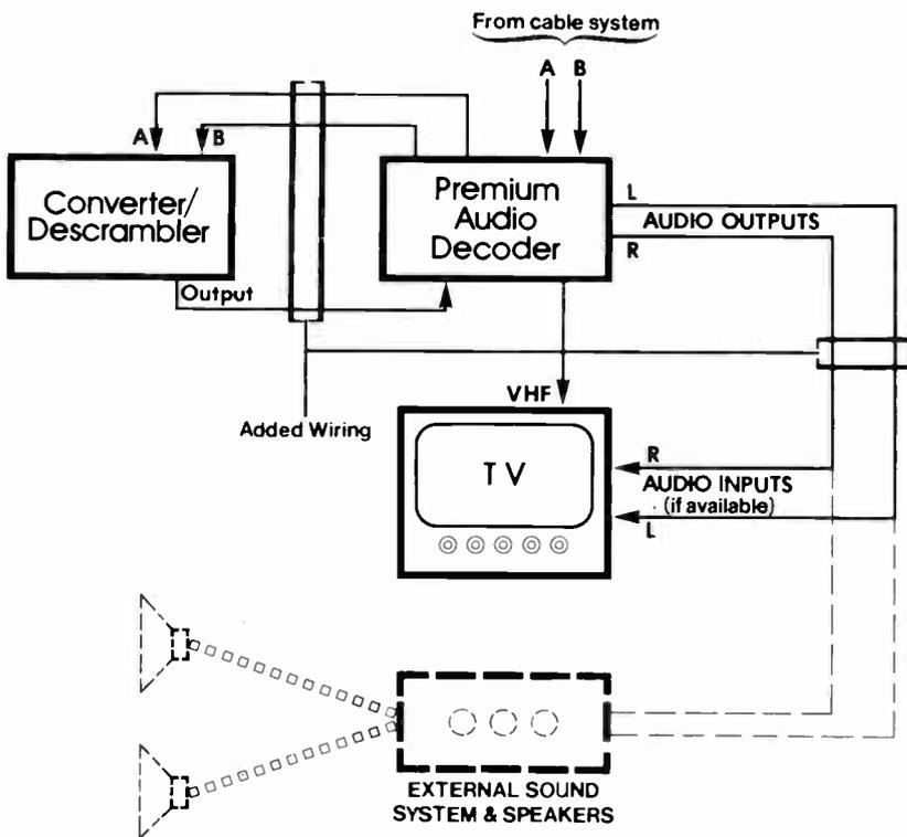
Figure 4 Typical Installation of Out-of-Band Stereo Decoder
