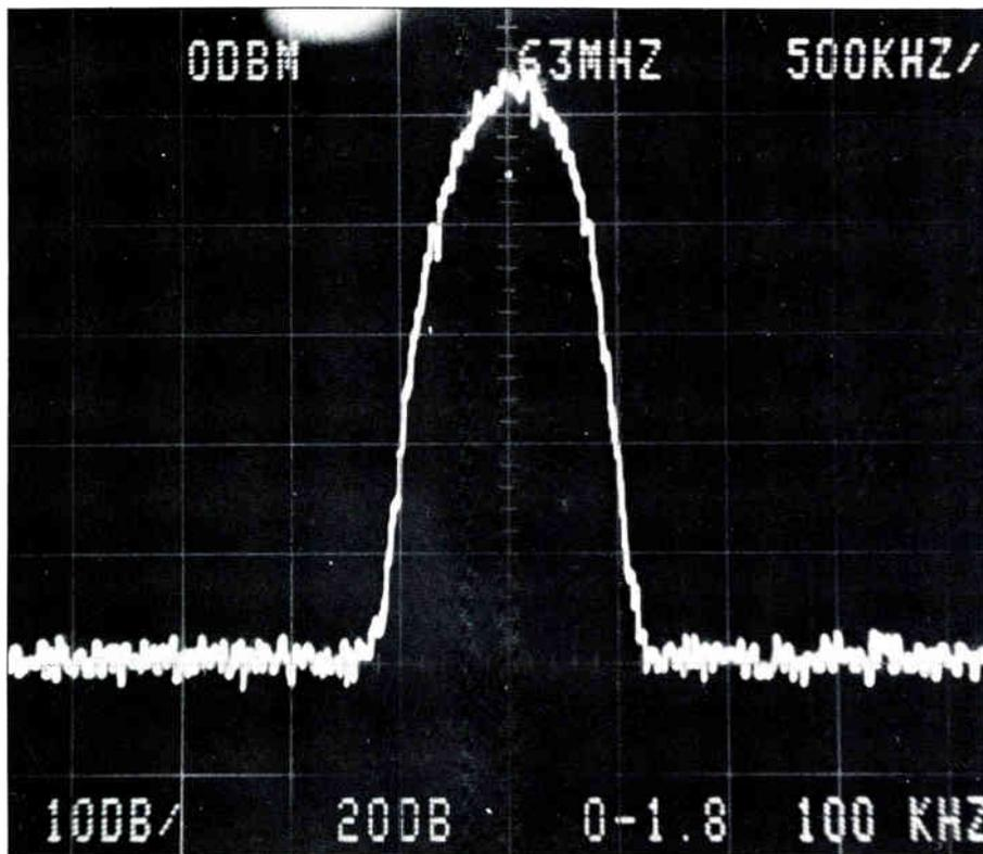
**Figure 1 Four-VSB frequency spectrum**
