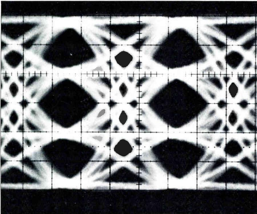
**Figure 2 Four-level eye pattern**
