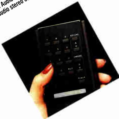
Channel mapping capability provides the cable operator with greater flexibility in TV and FM channel selection and programming. Use of an EEPROM gives the SM 2001 its impressive compatibility characteristics. The unit can be reprogrammed to tailor the system's mapped channels, and matching the converter output channel. Among the outstanding functional features of the SM 2001 are:
