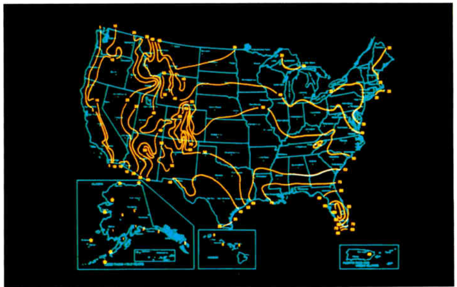
Iso-Keraunic map of the U.S. shows mean annual number of days with thunderstorms.
