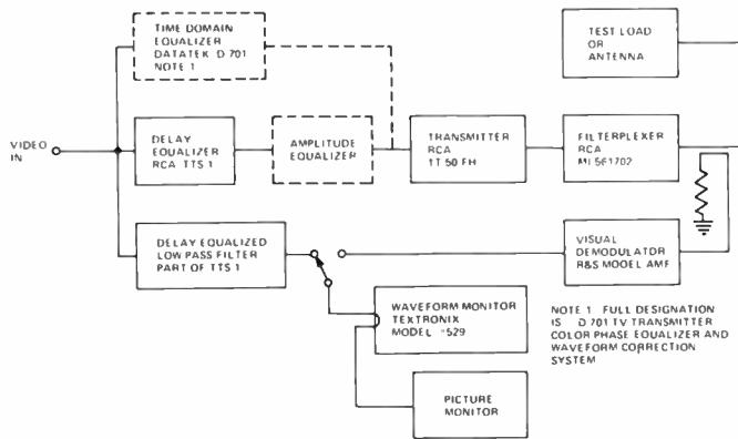
Figure 1 Block diagram of arrangement for evaluating TV transmitter transient response.
