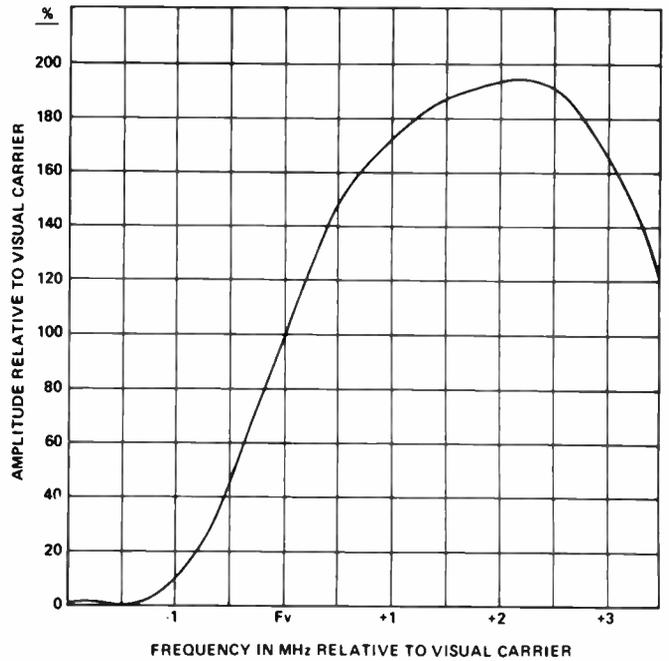
Figure 12 RCA color receiver RF-IF attenuation characteristic. Composite of one sample each of models: CTC-12, CTC-17, CTC-25, CTC-39, CTC-49 and CTC-60.
