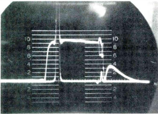
Figure 3 Transmitter sideband response associated with waveforms of Figure 2(a) and (b). Marker at 4.2 MHz. Notch at 4.5 MHz.
