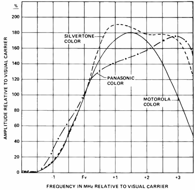
Figure 10 Standard (idealized) RA and TA characteristics, compared to demodulator attenuation tolerances and sample measurements.
