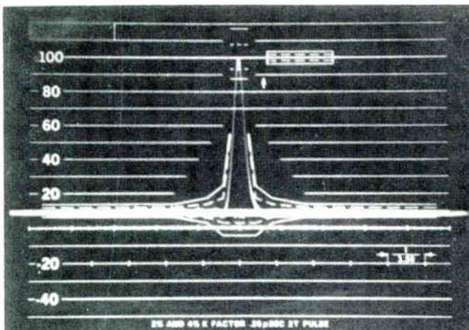
Figure 5 System response to 2 *T* sine-squared pulse. Transmitter adjusted in the time domain. Compare to Figure 2(a).
