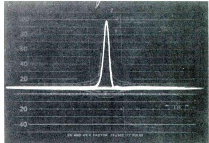
Figure 7 2 *T* sine-squared pulse response of system. Transmitter equalizer in frequency domain with Telemet 4501 demodulator.
