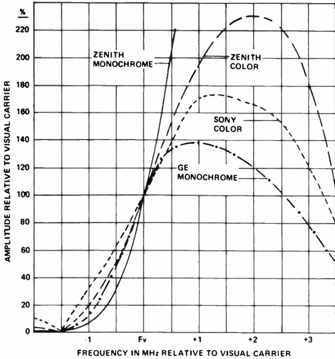
Figure 11b RF-IF attenuation characteristics of sample TV receivers<sup>1</sup>.
