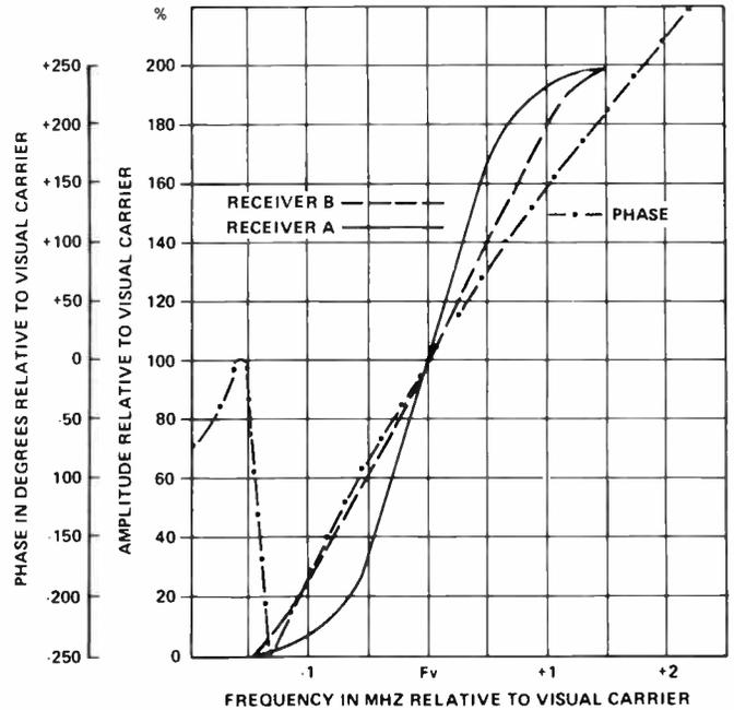
Figure 18 Attenuation and phase characteristics of representative receivers at extremes of lower sideband response.
