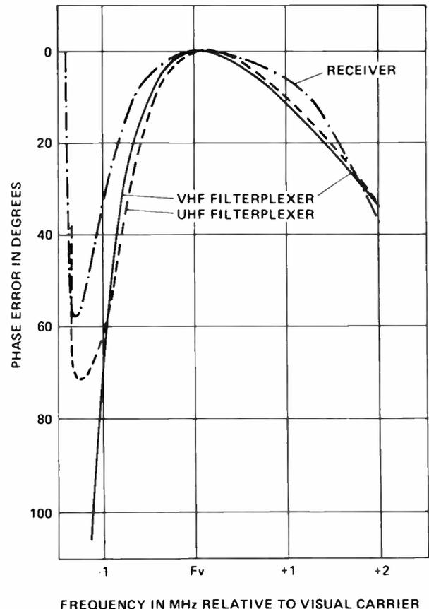
Figure 19 Transmitter (filterplexer) and receiver phase errors.
