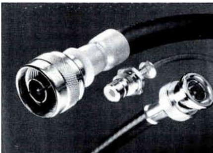
AMP Inc. introduced new cable-, panel- and bulk-head-mounted 75-ohm BNC, SNB and N-Series coaxial connectors for network applications up to 2 GHz. The connectors exhibit a VSWR of less than 1.3 and RF leakage less than -55 dB (-90 dB for N-Series). Hand tools or automatic machines may be used to apply the connectors.
