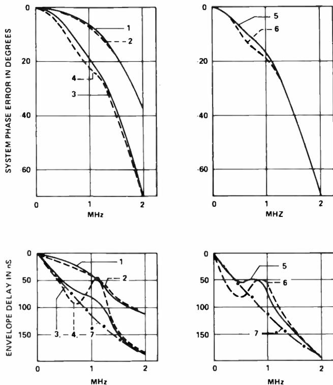
Figure 21 System phase and delay errors. Combinations of receivers and filterplexers. 1—receiver A and double sideband transmitter; 2—receiver B and double sideband transmitter; 3—receiver A and VHF filterplexer; 4—receiver B and VHF filterplexer; 5—receiver A and UHF filterplexer; 6—receiver B and UHF filterplexer; 7—appropriate transmitter delay equalization but invert slope.
