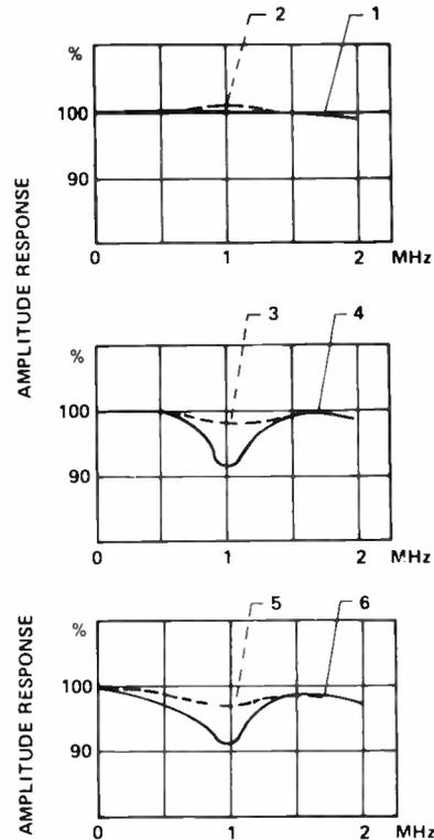
Figure 20 System amplitude versus frequency response for various combinations of receivers and filterplexers. 1—receiver A and double sideband transmitter; 2—receiver B and double sideband transmitter; 3—receiver A and VHF filterplexer; 4—receiver B and VHF filterplexer; 5—receiver A and UHF filterplexer; 6—receiver B and UHF filterplexer.
