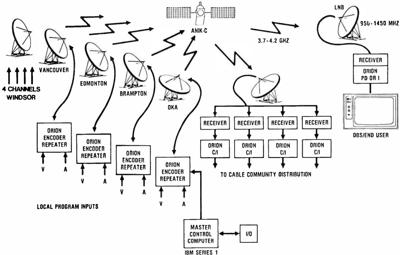
The flexibility of the ORION-NET system can be used to expand the dual system into a three-way system. The same signals can be carried through a CATV system without decoding and re-encoding. (See related article, *CED*, November 1985, pp. 16-26.)
