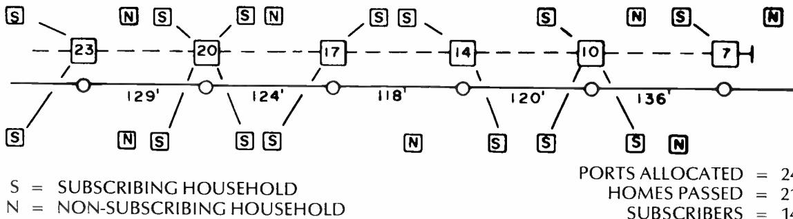
**Lower tap losses.** This particular example shows a loss of 1.2 dB per TGT or 4.8 dB passive loss. The traditional passive losses in Figure 1 total 8.6 dB without the terminating 7 tap! This increases the efficiency of line extender use in the system.
