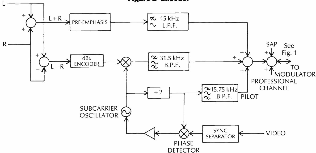
locked to the video horizontal line rate is transmitted. This pilot is doubled (usually in a phaselocked loop) and synchronously detects the L-R signal. As shown in the appendix, phase errors in the pilot result in amplitude errors in the recovered L-R signal. This, in turn,
