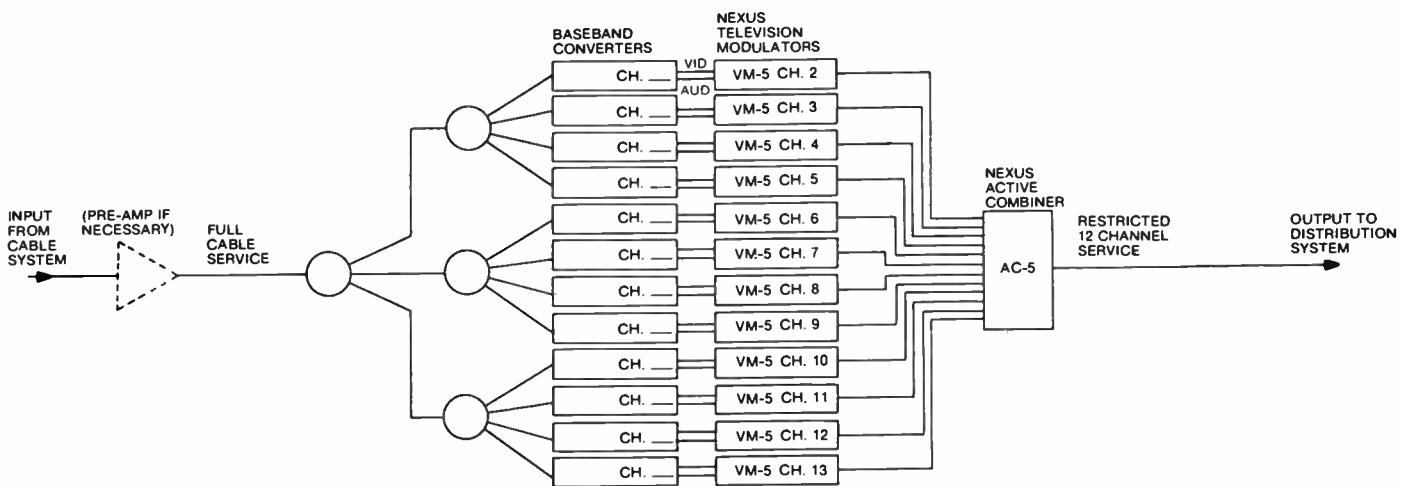
unscrambled cable signals because it is so economical. The set-top descramblers are very inexpensive and function well as demodulators. Good quality adjacent channel commercial modulators, for example, are now surprisingly affordable. This combination provides an agile input, adjacent channel output, demod-remod processor.
