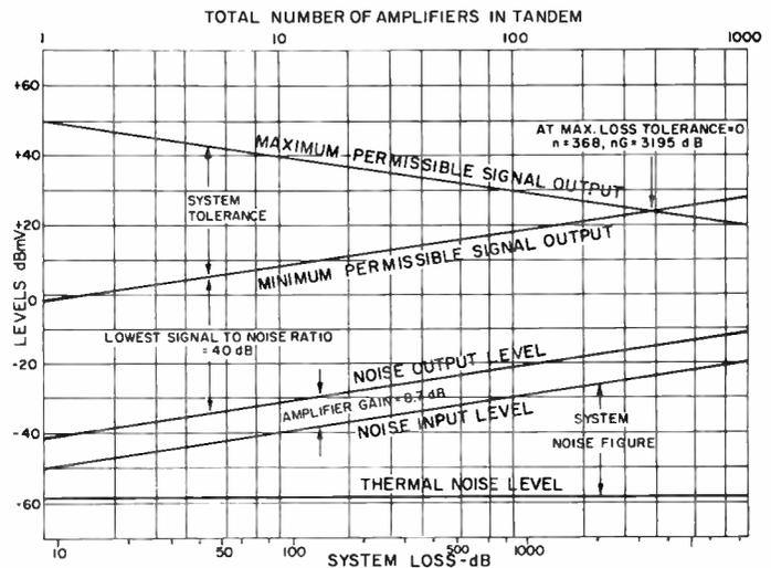
Figure 1. System level and tolerance diagram. Amplifier gain 8.69 dB. Output capability 50 dBmV. Noise figure 9.2 dB. Signal-to-noise ratio 40 dB.
