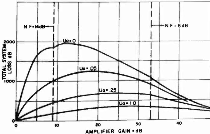
Figure 4. Achievable system loss versus amplifier gain for various "uncertainty" figures showing the effect of the assumed variation of noise figure with gain. Compare with Figure 2.
