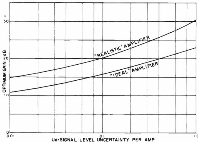
Figure 5. Variation of optimum gain with level uncertainty for the idealized amplifier and when the noise figure is a function of gain.
