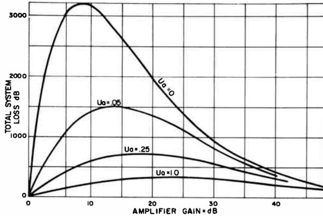
Figure 2. Achievable system loss versus amplifier gain for various "uncertainty" figures. The idealized amplifier has the same parameters as in Figure 1.
