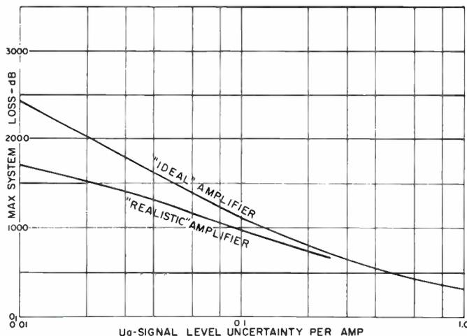
Figure 6. Variation of the maximum system loss with level uncertainty for the same conditions as in Figure 5.
