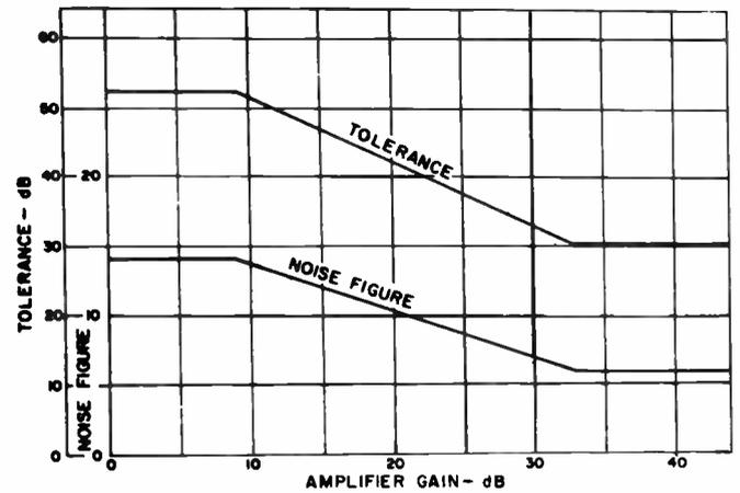
Figure 3. The assumed variation of noise figure with gain and the resulting variation in tolerance.
