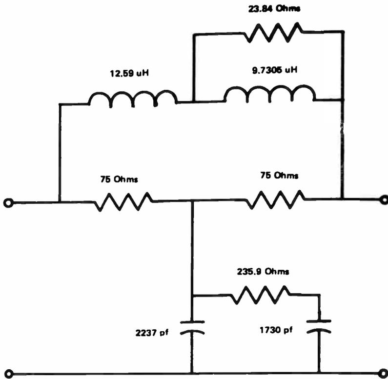
**Figure 4 CCIR noise weighting network**
