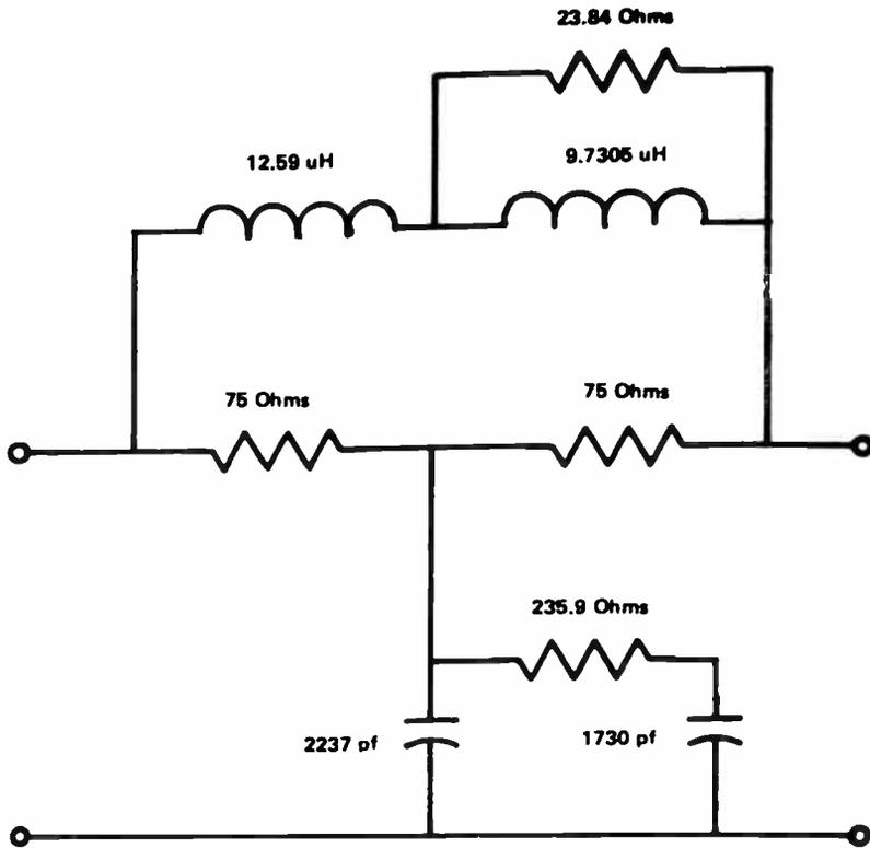
**Figure 4 CCIR noise weighting network**
