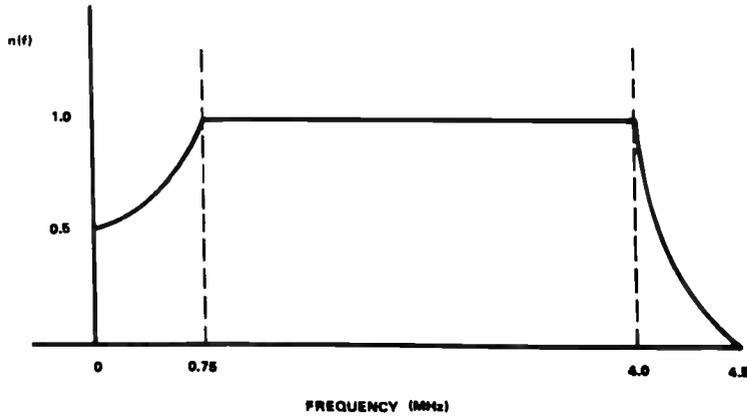
**Figure 6 Detected noise spectral density**
