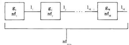
When the cable loss equals the gain, then  $g_k l_k = 1$  (where  $k = 1, 2, \dots, M$ ) and equation (8) becomes
