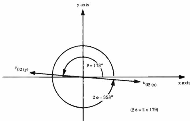
shows the improvement ( $I_{pp}$ ) due to push-pull versus the output inverter phase shift ( $\theta$ ) for various values of  $\phi$ . As can be seen from these curves, there are many combinations of  $\phi$  and  $\theta$  which yield perfect cancellation. A vector presentation of this mechanism is shown in Figure 10. From Figure 9, it is seen that for  $\Delta = 0$  dB, 20 dB of second-order reduction is possible with a phase unbalance as high as  $10^\circ$ .
