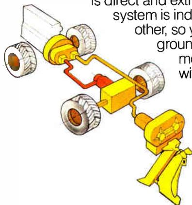
ground speed to accommodate soil conditions without disturbing your plow or chainline speed — or vice versa.
