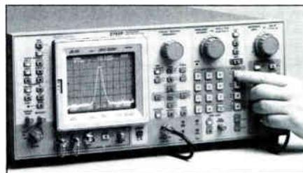
*Tektronix 2700 series spectrum analyzer*
