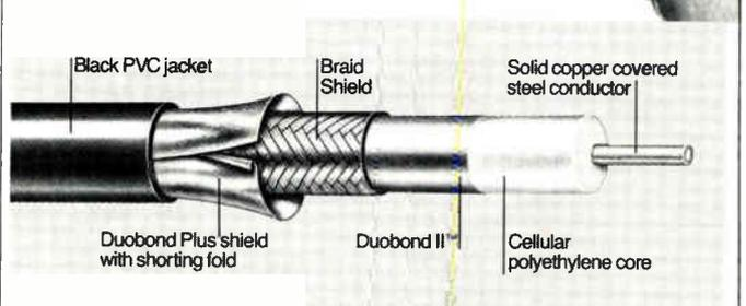
The inner foil of the DUOBOND PLUS shield is bonded *directly* to the core. Foil pushback and signal leakage problems are eliminated. Protection from shielding degradation is eliminated during installation—where most shielding problems occur.
