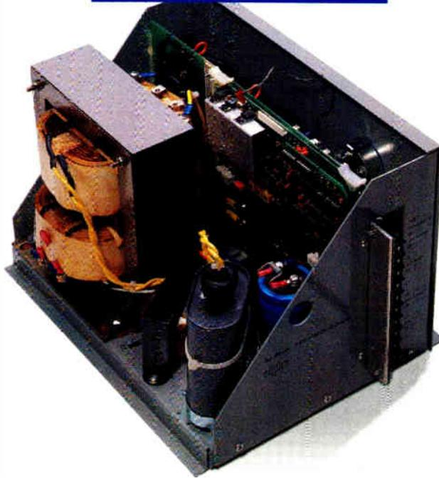
Pull off our cover and you'll see why Alpha is the CATV Standby Power Supply leader. Sure, we could have designed a system using two transformers like most manufacturers, but no, we decided that a single ferro-transformer would be more reliable. It was gutsy, it was innovative, and it works.
