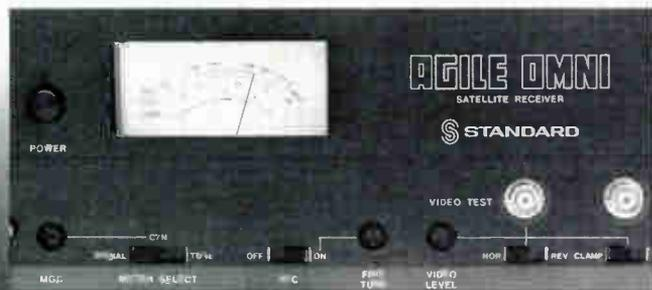
Operating functions including MGC, AGC, AEC, level sets, normal/invert video, clamp/unclamp video, skew, subcarrier frequency selection, video and IE test points are conveniently located on the main panel. Meter reads C/N ratio, signal strength or center-tune.
