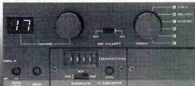
Format control enable selections of desired satellite system. Direct-reading channel selector displays transponder-assigned channel. Second selectable subcarrier and spare for optional third subcarrier or descrambler modules.
