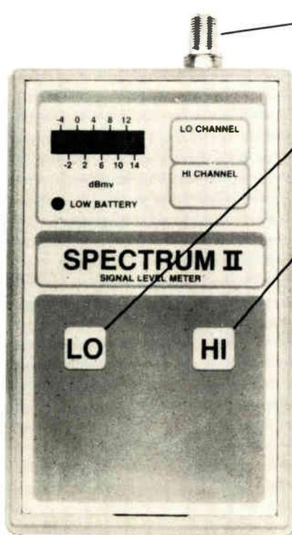
1. Connect the Spectrum II to the cable drop.
