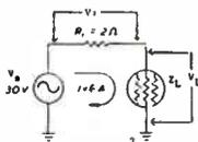
$$\begin{array}{lll} W = I^2R & V_1 = IR_1 & V_L = V_s - V_1 \\ W = 6^2(2) & V_1 = 6(2) & V_L = 30 - 12 \\ W = 72 & V_1 = 12 & V_L = 18 \end{array}$$
