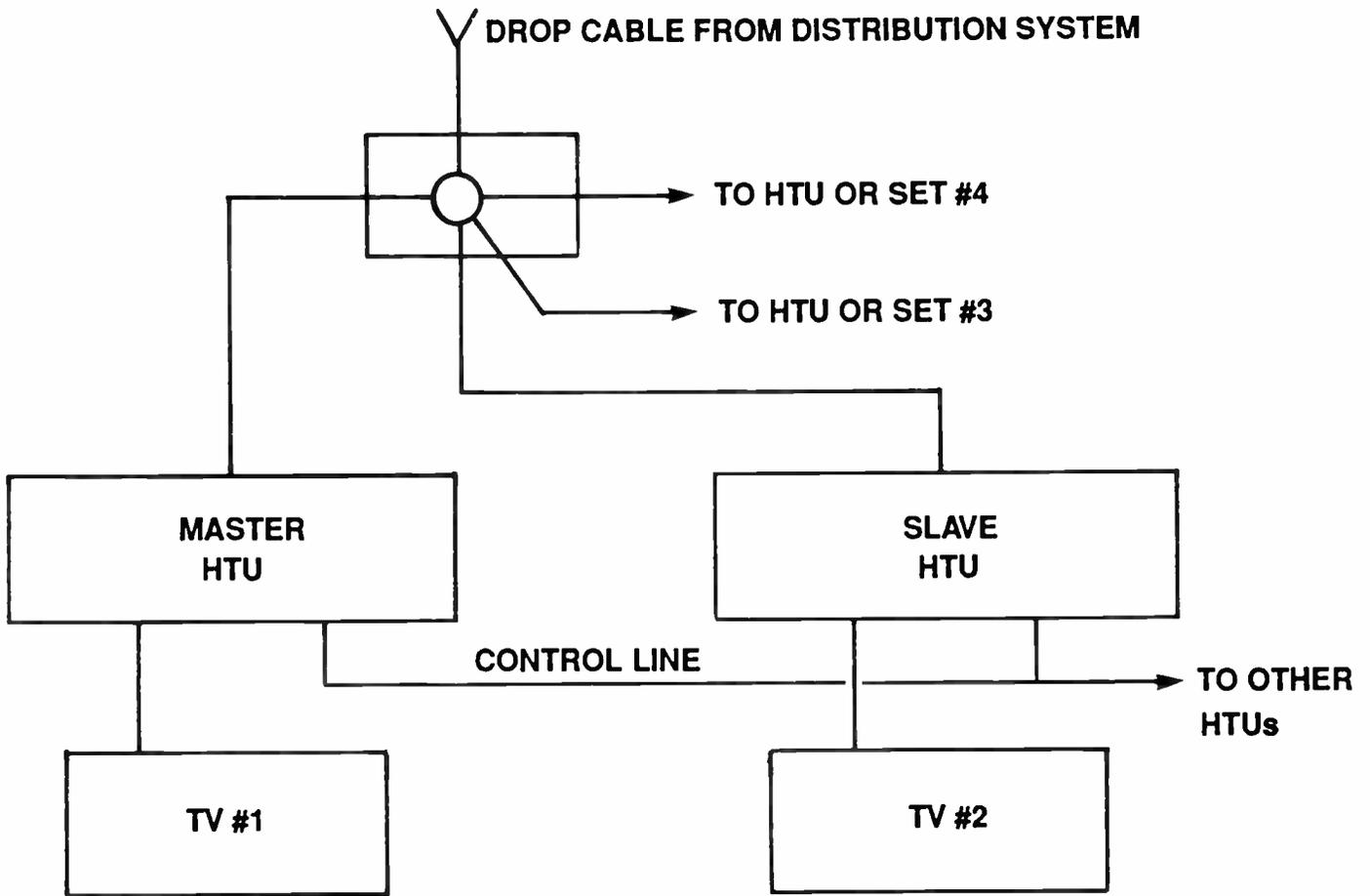
**Figure 2. Separate master-to-slave control line**
