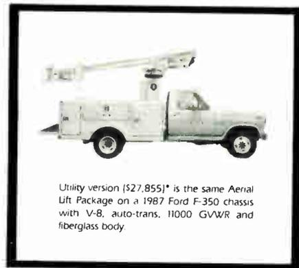
Utility version (\$27,855)\* is the same Aerial Lift Package on a 1987 Ford F-350 chassis with V-8, auto-trans, 11000 GVWR and fiberglass body.
