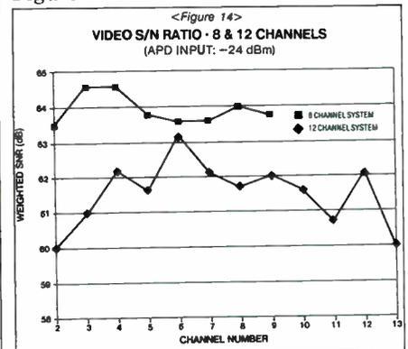
increased channel loading decreased video SNR performance somewhat, the same practical threshold was observed in terms of APD input, regardless of channel loading, at approximately -34 dBm. These tests were conducted by inserting additional attenuation at the end of the 20.9 dB fiber path. The system as configured, with a laser output of -2.7 dB, has a maximum path loss to threshold of 31.3 dB. This figure is higher than expected and speaks
