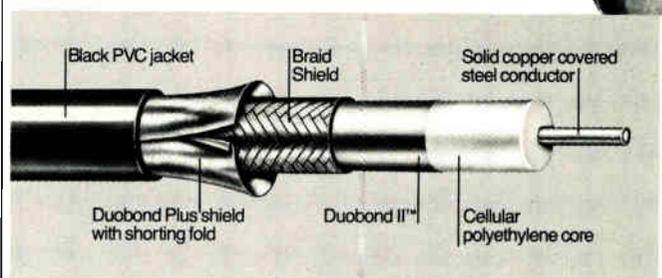
The inner foil of the DUOBOND PLUS shield is bonded *directly* to the core. Foil pushback and signal leakage problems are eliminated. Protection from shielding degradation is eliminated during installation—where most shielding problems occur.
