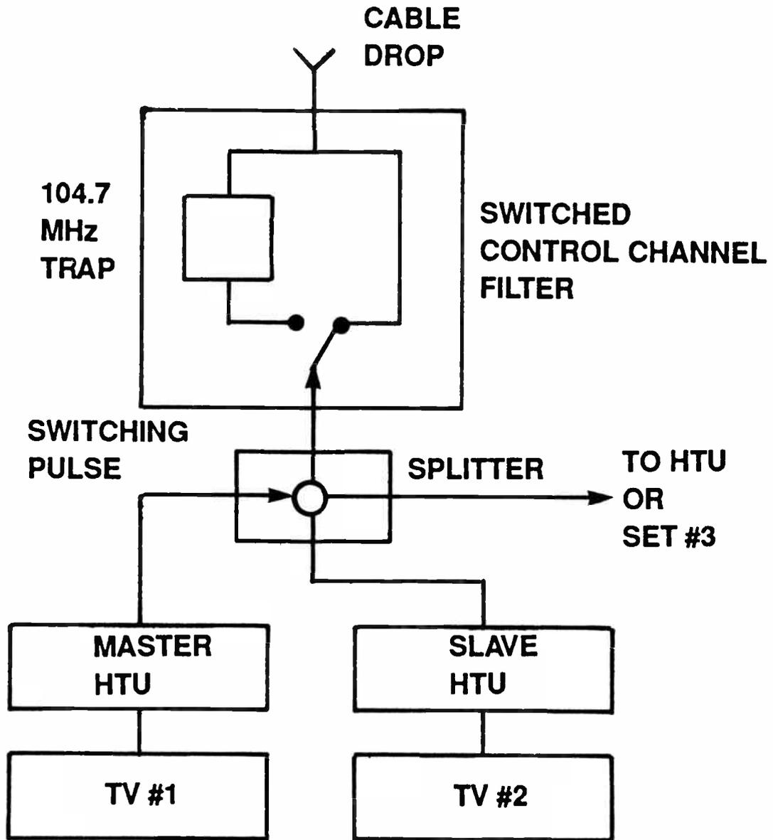
**Figure 3. Control channel interrupt**
