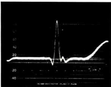
Multiburst and 2T Pulse Response — 6300 Modulator — TV Receiver
