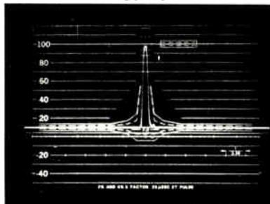
"Character Generator Pulse" — 75 Nanosec Wide — 15 Nanoseconds Rise and Fall Times
