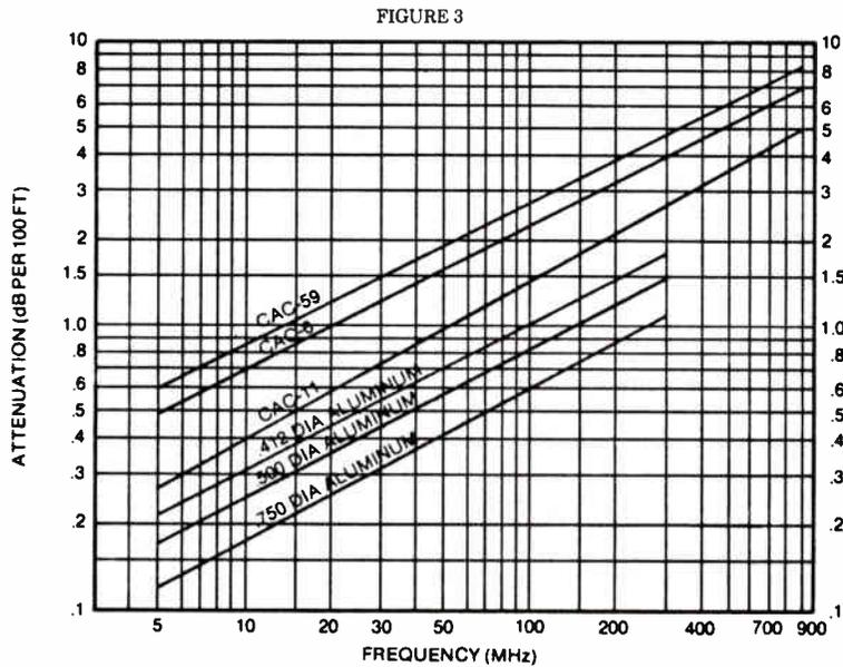
Cable Attenuation Versus Frequency for Various Sizes of Coaxial Cable
