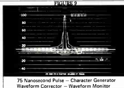
This paper describes a technique whereby the overall system transient response is improved by altering the system characteristics in the time—domain. In our example, the output of the character generator has been pre-distorted before going to the modulator by adding in a correction signal which
