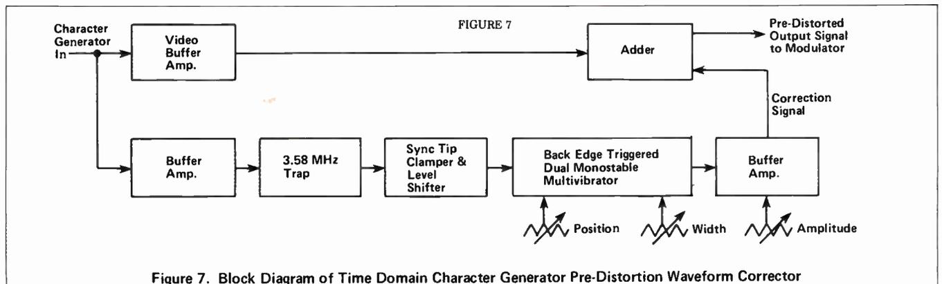
Figure 7. Block Diagram of Time Domain Character Generator Pre-Distortion Waveform Corrector
