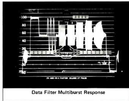
backgrounds became popular, these filters were rendered useless because of the loss of color saturation they produced. Further attempts to design data filters produced results such as that shown in Figure 7.
