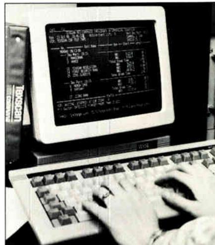
*Texscan's MSI Compuvid* random access or full random access modes. Printer output is available for logging and verification. Several levels of traffic and billing systems are available, and printouts include verification of good video. All Comserter models are capable of remote control of many headends and can be mixed and matched to expand system capabilities.
