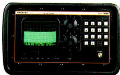
Now you can change sweep center frequency and span from the field. Use a vertical marker in "sweepless" mode to identify and zoom in on a response problem. Then, at the same setting, quickly switch to the spectrum analyzer
