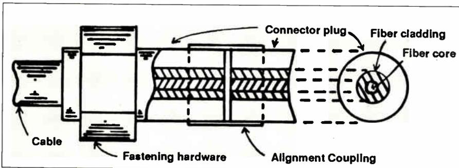
However, there are many fiber optic connectors available today that can easily and consistently achieve and maintain good optical alignment, at low cost. One needs only to be careful when selecting an optical connector. In most respects, optical connectors can be handled in the same way as connectors used with metallic media (e.g., coax). Optical connectors must, however, be kept clean.
