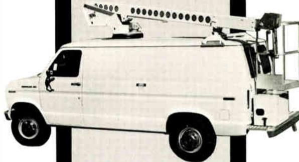
A-28 van mounted lift with APU. Utility-body mounted lift also available.
