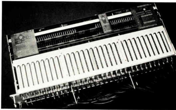
*A Mk 1 switch unit, capable of serving 30 customers.*
