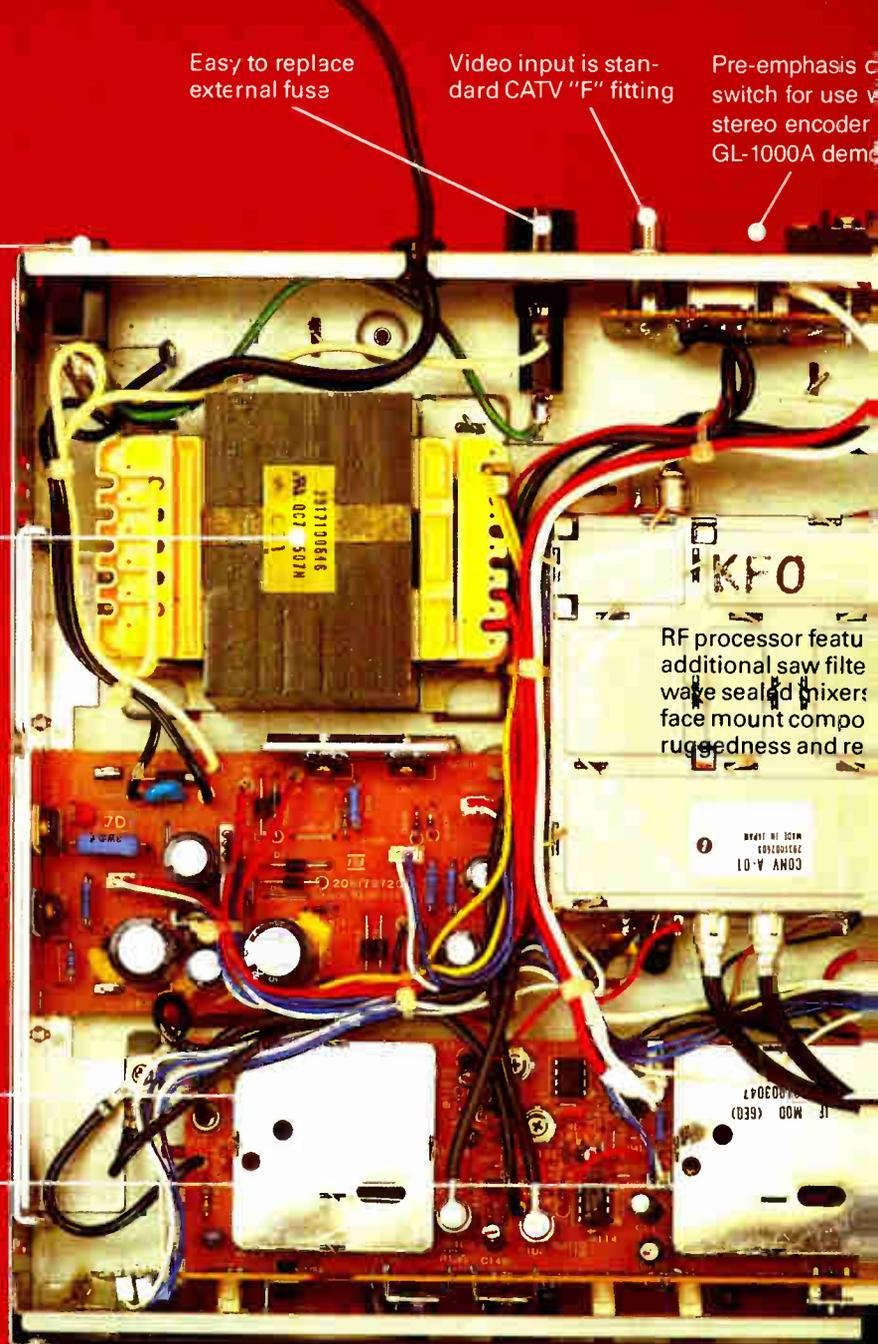
RF processor features additional saw filter, wave sealed mixers, face mount components, ruggedness and reliability.
