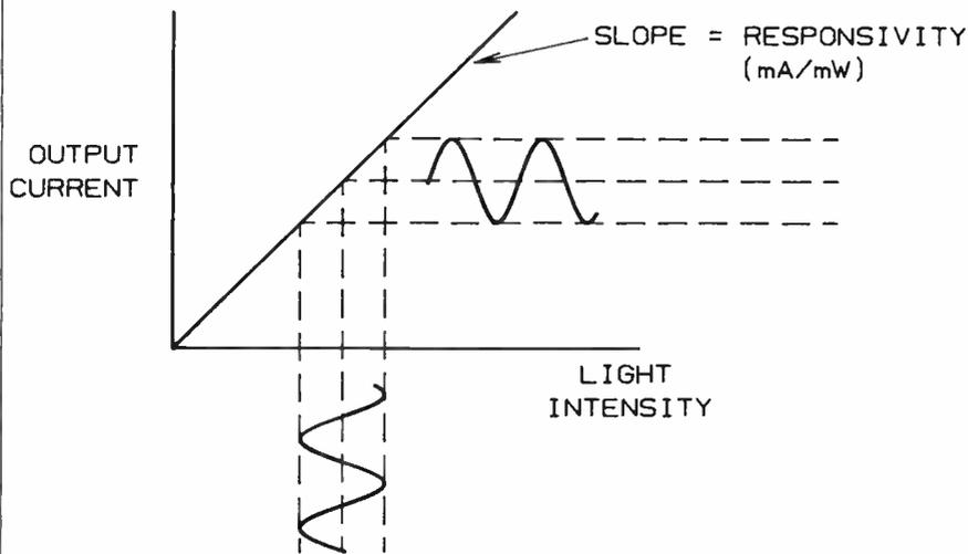
Fundamentally, a photodiode converts photons (light) into electrons (current) with excellent linearity and virtually no excess noise. Figure 3 shows the process by which analog signals are generated from an input optical signal.
