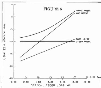
optical signal produces a DC photocurrent that has an accompanying shot noise. Paradoxically, proper system design favors high received optical power to minimize the effects of shot noise. Although this actually increases the
