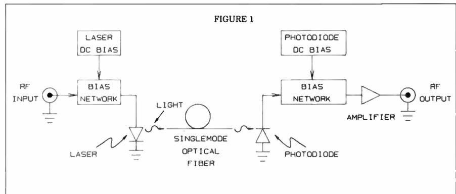
input connector is particularly useful in high frequency analog systems. Also very important is an internal matching resistor to build the laser dynamic resistance up to 50 or 75 ohms, depending on the application.
