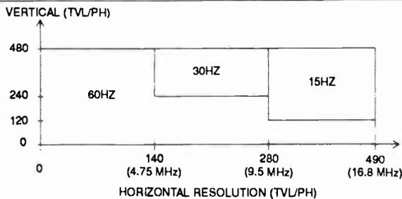
To conserve spectrum the N.A. Philips MAC System transmits only a portion of the contents of some lines by first using a low pass filter. The table shows the resolution of each luminance and color-difference line. This pattern repeats every 8 lines. The luminance pattern moves up one line every frame. The color-difference signal pattern moves up two lines every frame. The signal is 525 line progressive scan. The resulting luminance temporal-spatial resolution is also shown.
