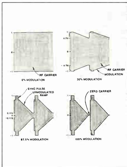
course, some modulators do offer modulation meters that are useful, and for a more exact measurement, a spectrum analyzer, or a TV demodulator with a "zero chopper" (zero carrier reference) along with an oscilloscope, can be used to monitor the depth of modulation.
