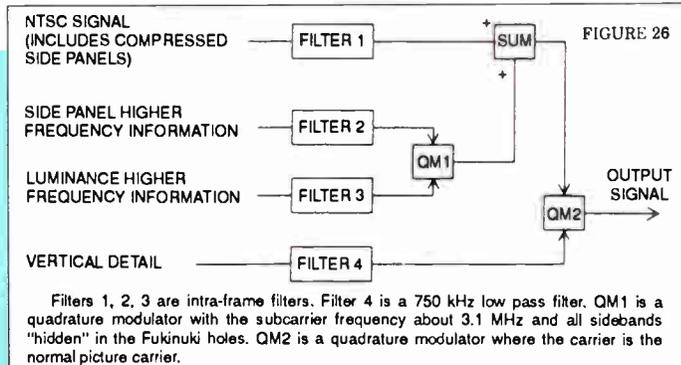
**Signal encoder block diagram—NBC**
