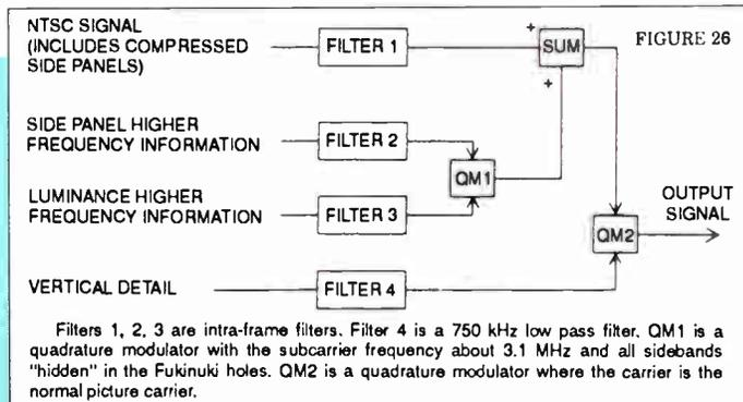
Filters 1, 2, 3 are intra-frame filters. Filter 4 is a 750 kHz low pass filter. QM1 is a quadrature modulator with the subcarrier frequency about 3.1 MHz and all sidebands "hidden" in the Fukinuki holes. QM2 is a quadrature modulator where the carrier is the normal picture carrier.
