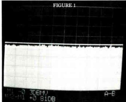
Normalized high level response at headend test point. Comparison between the high level sweep (Wavetek 1855B/1865B) and the Sweepless Sweep® analysis.
