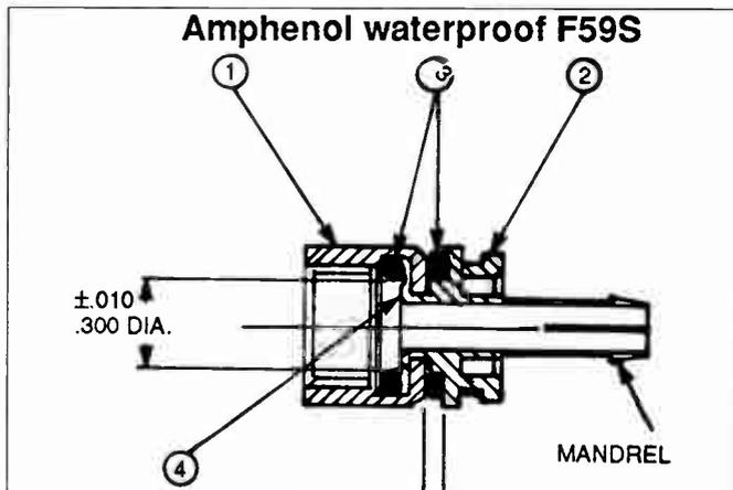
Electronics developed a solderless and easy to install connector called the F59.
