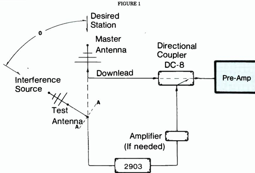
insert a pay-TV negative trap corresponding to the offending channel between antenna and pre-amp (or processor, if there is no pre-amp). This works well for all off-air channels if the offending channel is below the desired one: the trap gives little loss to the desired video carrier. If the offending channel is above the desired one, such traps will attenuate the desired audio carrier. This is usually tolerable for
