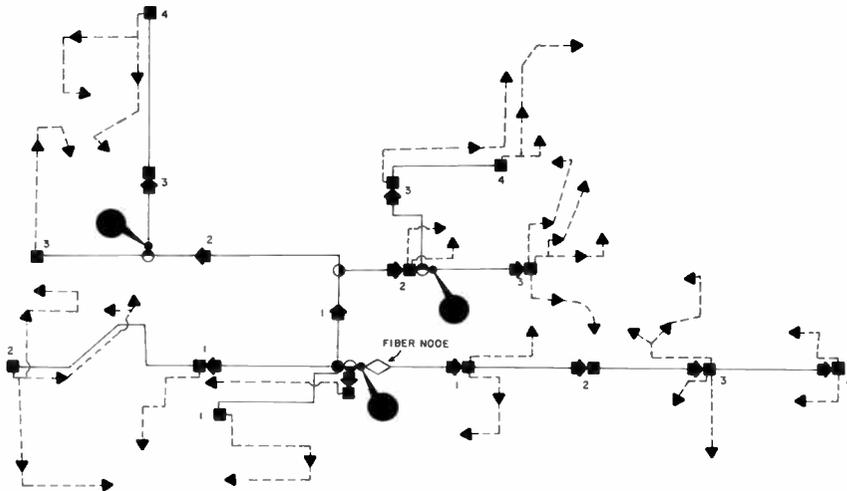
EXHIBIT 11, TYPICAL TRUNK DIAGRAM FOR FIBER NODE PLUS FOUR IN CASCADE
