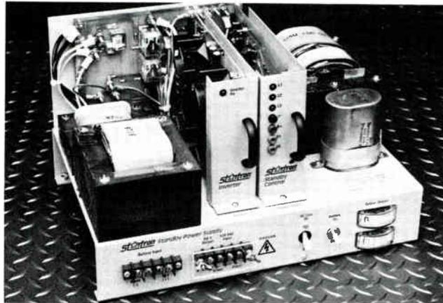
common sense approach you get a standby supply that keeps working long after others fail as each critical circuit is protected by a high speed MOV. With multiple MOVs we're serious about protecting more than just a warranty.
