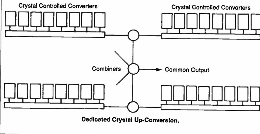
**T**wo different design concepts for new headend construction or channel addition are available today: non-modular (no front panel modules) frequency agile up-conversion (FAC); and front panel modular, dedicated crystal up-conversion (DCC).
