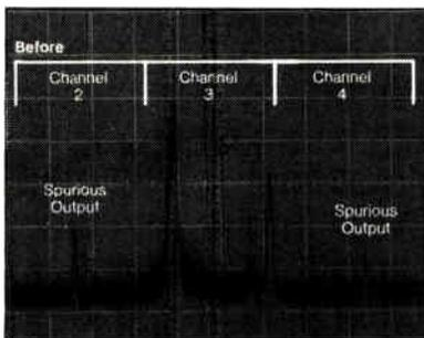
Spectrum of channel 3 modulator direct output showing spurious outputs into adjacent channels
