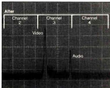
Channel 3 modulator spectrum filtered through a bandpass filter. Adjacent interference is removed
