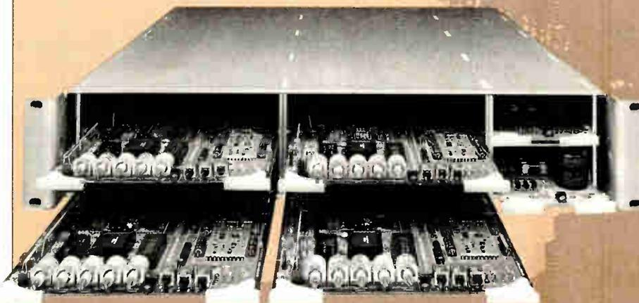
The new 7510 video processing amplifier from the Grass Valley Group is designed to process "off air" signals from satellites, microwaves and land lines.
