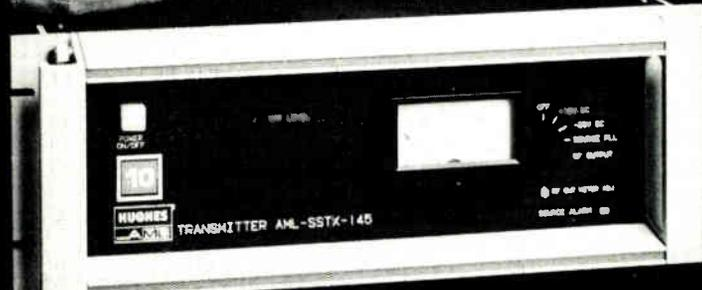
the new transmitter is also compatible with that of the STX-141, making it possible to expand existing arrays previously limited by floor space or prime power considerations. What's more, when used in conjunction with our new CORE 3-299 receiver, you'll be able to demonstrate an 80-channel microwave system with better than 58 dB C/N and 65 dB C/CTB—even when all receivers are more than 20 miles distant.
