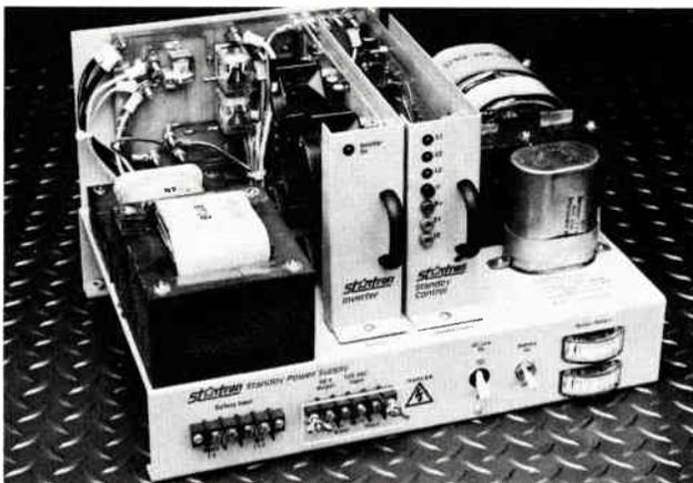
common sense approach you get a standby supply that keeps working long after others fail as each critical circuit is protected by a high speed MOV. With multiple MOVs we're serious about protecting more than just a warranty.
