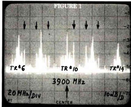
When pointing the dish toward a satellite, the transponders and the interference carriers are clearly displayed on the screen of the analyzer. The vertical arrows mark the interference carriers.
