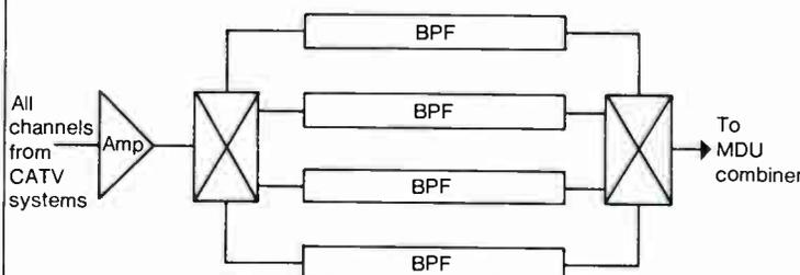
Figure 2: Deletion of channel for closed-circuit reuse
