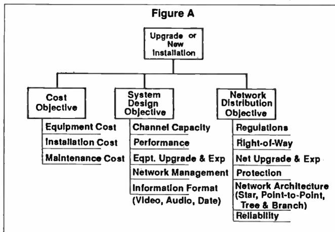
lation are: property acquisitions (right-of-way, pole space and tower sites), manpower, and construction permits and licenses. Maintenance costs involve test equipment, outside plant repair and service personnel.
