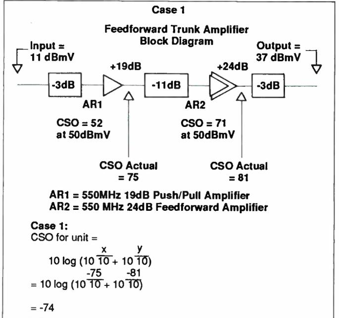
In order to see the effects of CSO on a CATV system, models of these amplifiers will be made using the average CSO numbers from Tables 1 through 3. In the case of the trunk amplifier a push/pull hybrid will be used together with the feedforward block. The bridg-
