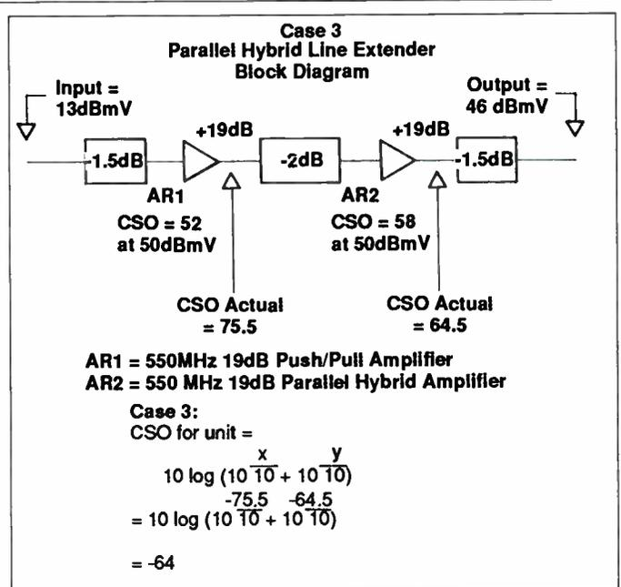
ing amplifier and line extenders will both be parallel hybrid units, meaning that the push/pull hybrid will be used as the input with the parallel hybrid device used as the output. Levels for the units will be +11 dBmV input; 37 dBmV output for the trunk; and the
