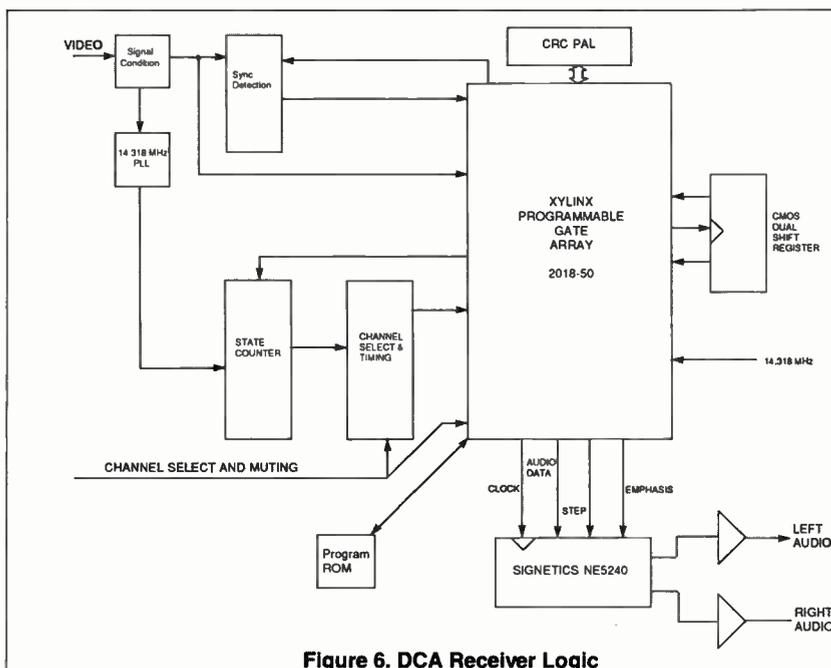
Figure 6. DCA Receiver Logic
