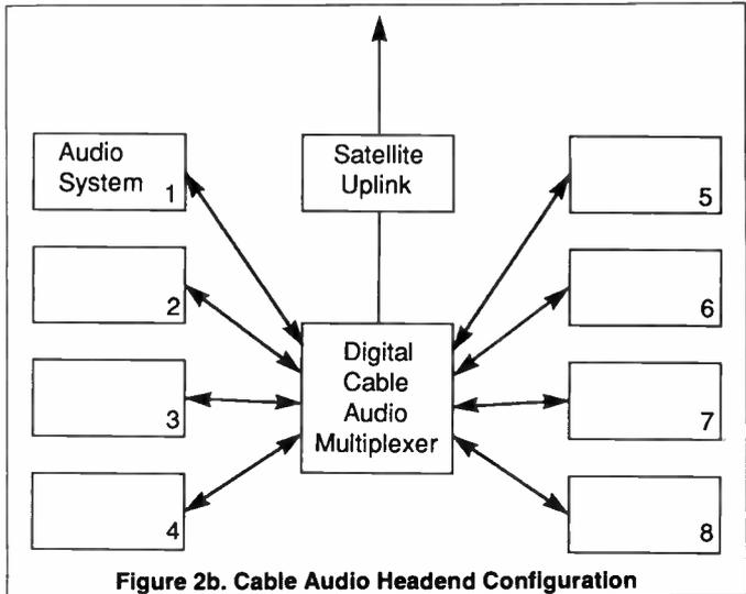
Figure 2b. Cable Audio Headend Configuration
