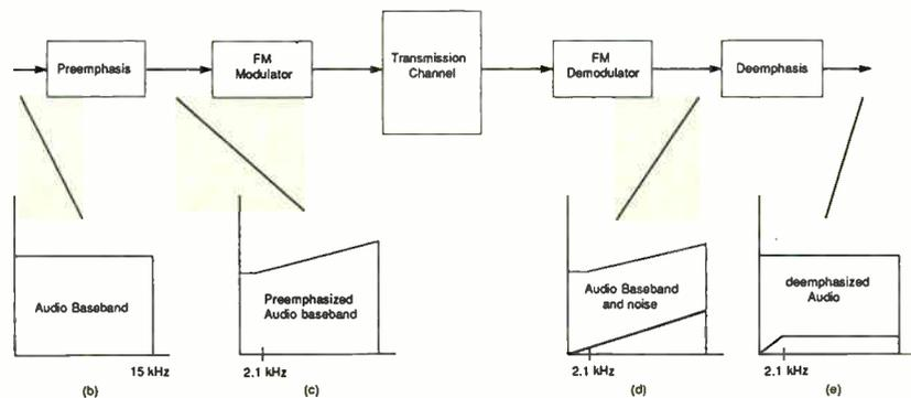
reducing the noise at the output of the discriminator by following it with a simple single-pole low-pass filter that would counteract the discriminator's rising output noise characteristic. The net result being a noise spectrum that is very nearly flat with increasing frequency. There is a slight problem with this approach however, because placement of a low pass filter following the discriminator also filters the mes-
