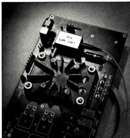
New Tektronix laser controller kit
