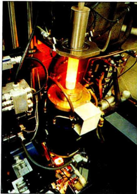
An outside vapor deposition blank is lowered into the draw furnace to begin the fiber drawing process.
