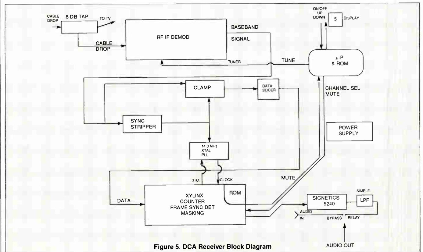
Figure 5. DCA Receiver Block Diagram
