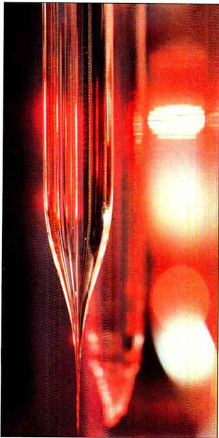
A partially drawn outside vapor deposition blank is displayed to demonstrate how a blank is drawn down to fiber.
