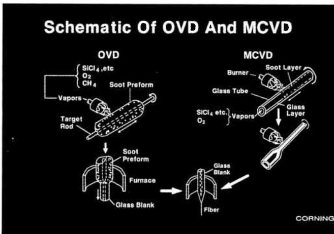
that eventually becomes an integral part of the finished fiber. The most commonly used IVD process is the Modified Chemical Vapor Deposition (MCVD) process. In this method, a glass tube is placed in a lathe and rotated while a burner flame traverses back and forth along the length of the tube to heat it.
