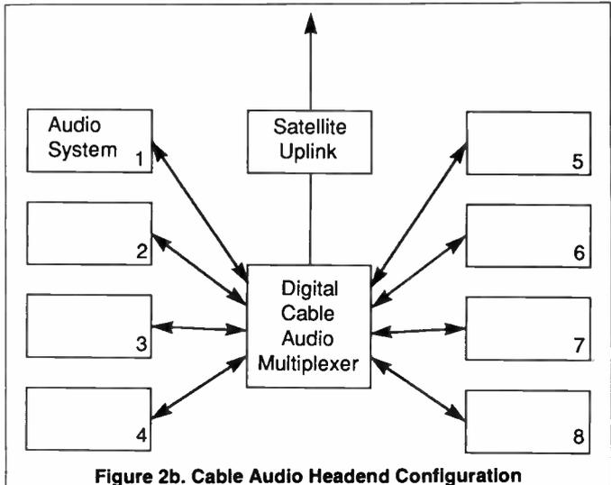
Figure 2b. Cable Audio Headend Configuration
