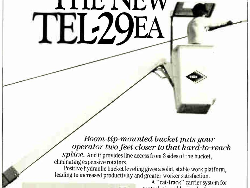
*Boom-tip-mounted bucket puts your operator two feet closer to that hard-to-reach splice.* And it provides line access from 3 sides of the bucket, eliminating expensive rotators.
