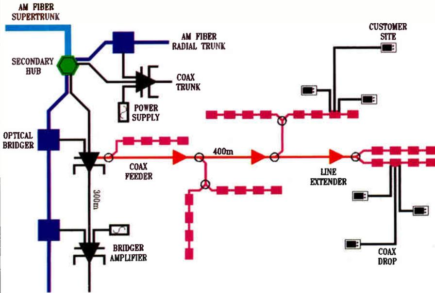
Figure 6. Hybrid fiber/coax topology
