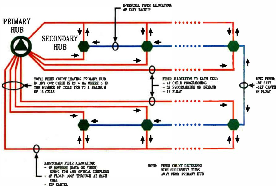
**Figure 3. Redundant ring connection of hubs**
