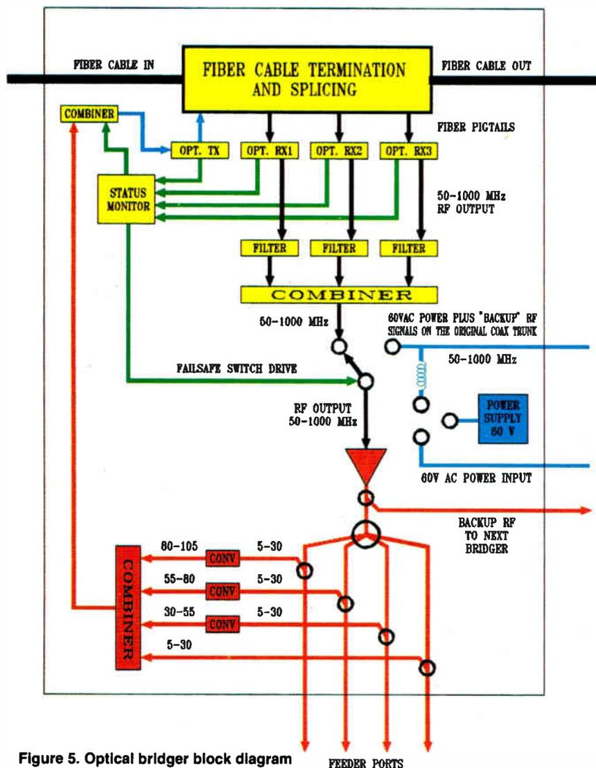
Figure 5. Optical bridger block diagram
