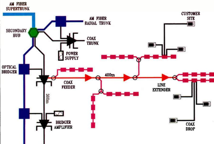
Figure 6. Hybrid fiber/coax topology
