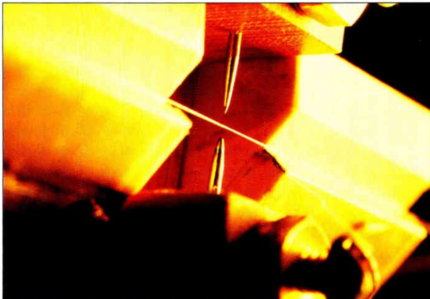
*Fiber undergoing fusion splicing*
