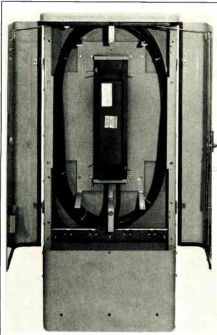
*Reliable Electric's fiber optic splice cabinet* signed to protect fiber optic splices in both burial and aerial distribution systems, the weatherproof cabinet includes the necessary hardware to mount most fiber optic splice closures. The fiber splice capacity is limited only by the size of the splice closure while cable management posts allow storage of up
