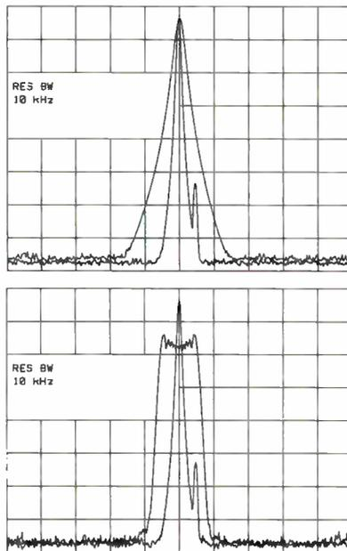
a) (above) Filter shape absorbing an adjacent signal
