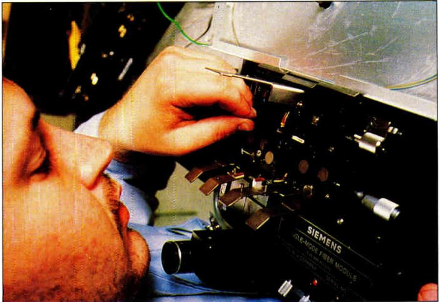
*An engineer feeds optical fiber into a fusion splicer*
