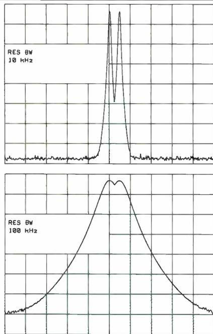
a) (above) Bandwidth less than signal separation
