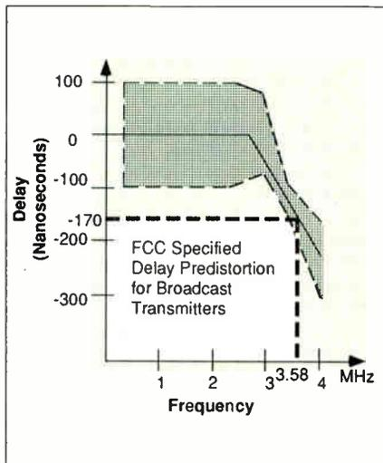
delay near the edges of its passband (read color subcarrier) relative to the center of its passband (read luminance).
