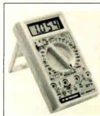
Called the Test Bench® Jr., the Model 377 is a smaller line addition to the Test Bench®. The Model 377 is a 39-range voltmeter/ammeter/ohmmeter/frequency counter/capacitance tester/logic tester/transistor tester/diode tester/continuity tester. It measures 5 inches by 2 7/8 inches by 1 3/8 inches and features the triple protection of reverse polarity protection, overload protection and high-energy fusing. For more info call, (312) 889-9087.
