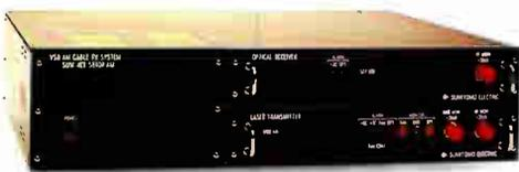
**RACK MOUNT.** Two half-height transmitter and/or receiver units are supported by a single 2RU chassis/power supply.
