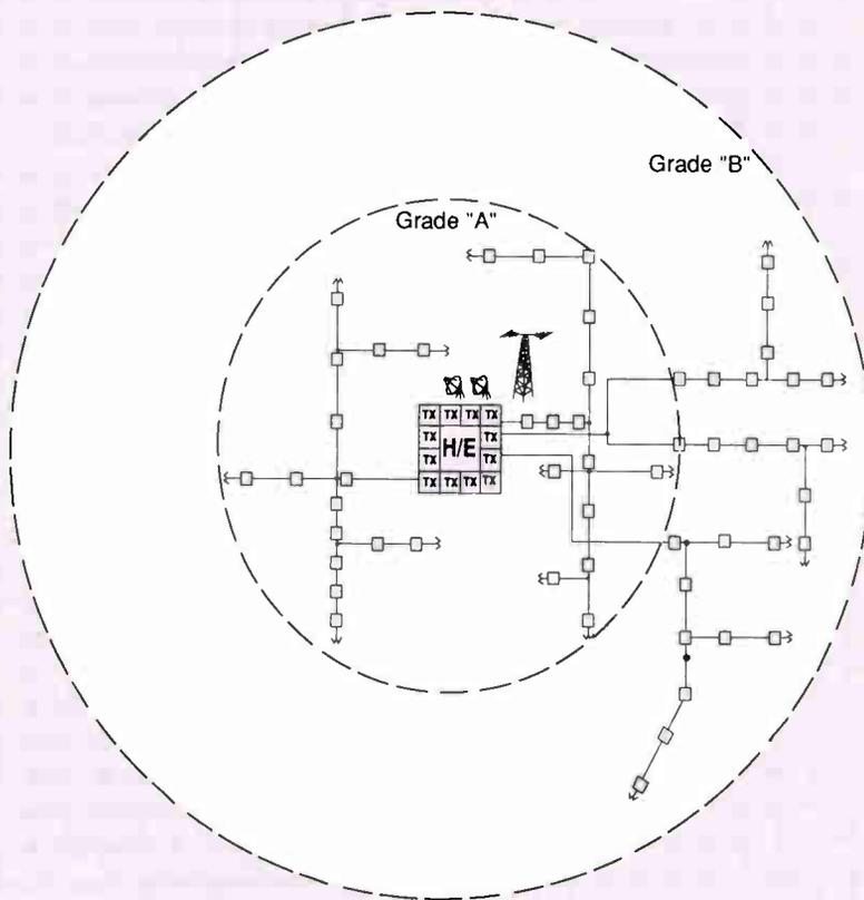
Grade contours represent a theoretical distance limit by which optical light sources may be split multiple times from a single source and deliver acceptable optical input signals to the receiver at each tap location. At each tap location, the light source is converted to RF energy to provide +15 dBmV to +20 dBmV at the subscriber port.
