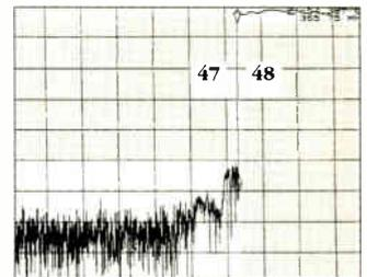
Brickwall HPF 6211HP-47/48 Passes Channel 80 Up, 50 dB Channel 47 Down
