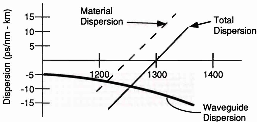
Total = Material + Waveguide
