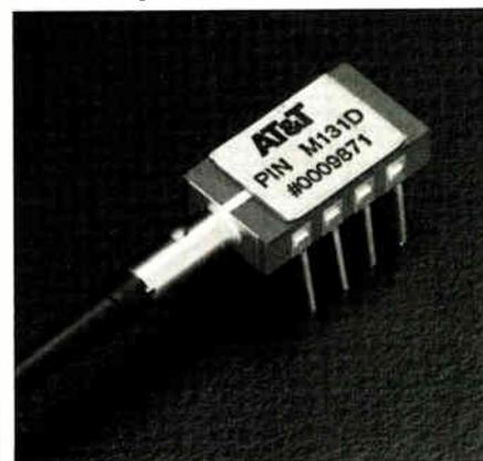
AT&T Microelectronics' 1310 Astrotec® long-wavelength PIN photodetector
