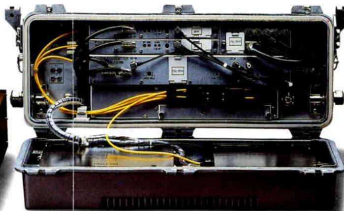
Our new, economical VSB-AM strand mount optical receiver frees you to create fiber-to-feeder and fiber-to-line-extender architectures.
