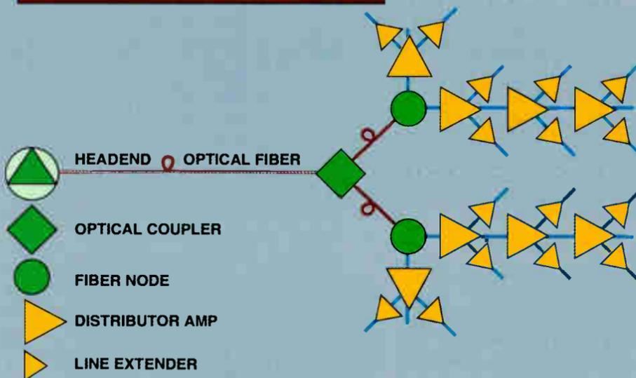
Optical coupler, and economical Sumitomo receiver serving as a secondary node, provide unprecedented network design freedom. Fiber-to-feeder architecture further reduces active cascades and reduces maintenance by eliminating RF trunk amplifiers.
