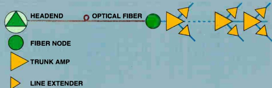
Conventional fiber backbone reduces active cascades as compared with coaxial trunk system. This improves picture quality and service reliability while extending system range. Sumitomo full bandwidth transmission and plug-in filters provide flexible split-channel loading. A/B switch provides system redundancy.
