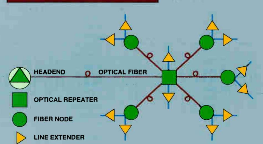
Sumitomo strand-mount optical repeater and secondary-node receiver eliminate need for trunk and distribution amplifiers. Resulting fiber-to-line-extender architecture minimizes active devices between headend and subscriber. Advanced design also minimizes maintenance, and allows expansion without backbone redesign or rework.
