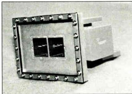
*Seavy Engineering's Multi-Sat 2° spacing* mode transducers which provide dual linear polarization on each beam. For more information, phone (617) 383-9722 or fax inquiries to (617) 383-2089.
