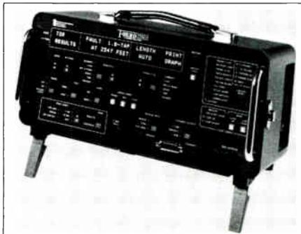
TTC's T-BERD 209A T-carrier analyzer new time domain reflectometer (TDR) identifies and isolates cable faults such as bridge taps, opens and shorts by indicating the fault type and distance
