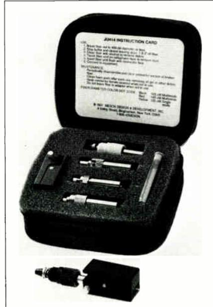
*Meson Design & Development's JU 414* assortment of multimode or single-mode connector modules, clean-out wire and a JU 414 adaptor body. The unit is designed for use in acceptance testing of fiber before and after installation, or any time there is a need to temporarily connect a fiber to an OTDR, power meter, light source or other equipment. For more information, phone 800-45-MESON or fax inquiries to (607) 722-3945.
