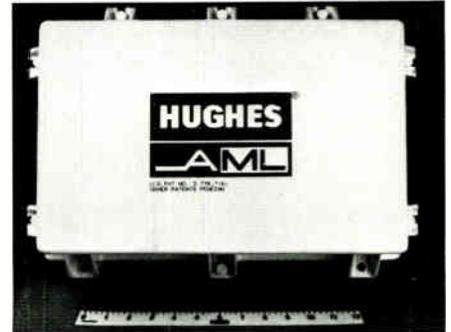
*Hughes' outdoor compact transmitter* highest power model, the HCOT-114, has the capability of transmitting 40 channels over one 20-mile link or four 10-mile links with 53 dB C/N and 65 dB C/CTB. The other units, each approximately three dB down from the next higher model, are the COT-113, the MCOT-120 and the LCOT-119. A built-in pilot tone generator in each unit is compatible with all Hughes phase-lock receivers. For more information, phone (213) 517-6233.
