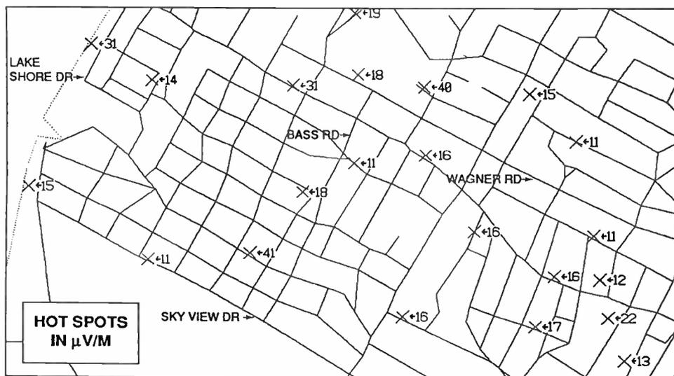
With the ICS LeakFinder™, your drive outs will be faster and cheaper. Until ICS created LeakFinder, drive outs did not produce maps. Technicians across the nation are finding that they can fix leaks more efficiently with the maps produced by LeakFinder than by lists of addresses.
