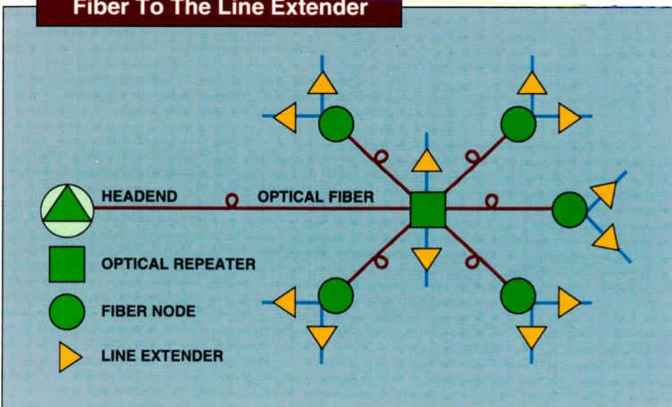
Sumitomo strand-mount optical repeater and secondary-node receiver eliminate need for trunk and distribution amplifiers. Resulting fiber-to-line-extender architecture minimizes active devices between headend and subscriber. Advanced design also minimizes maintenance, and allows expansion without backbone redesign or rework.
