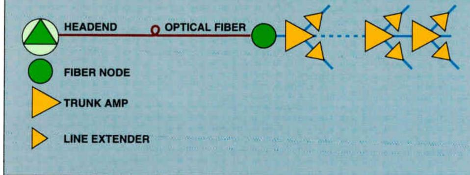
Conventional fiber backbone reduces active cascades as compared with coaxial trunk system. This improves picture quality and service reliability while extending system range. Sumitomo full bandwidth transmission and plug-in filters provide flexible split-channel loading. A/B switch provides system redundancy.
