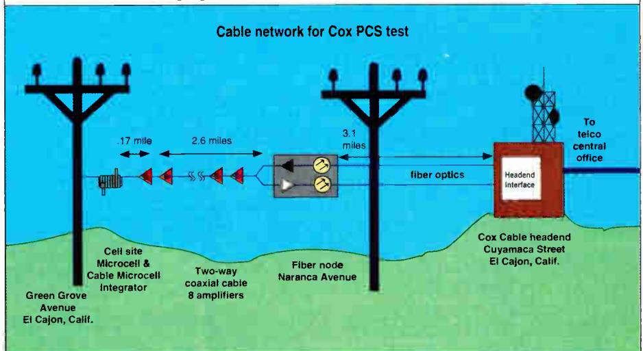
communicates through antennas with the hand-held portable phone. The integrator allows the microcell to be connected to the cable plant by combining digital voice signals from the radio equipment into a single high-speed digital signal.
