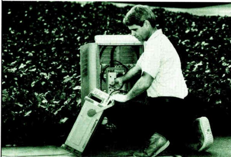
**HP's portable CATV analyzer speeds up troubleshooting.**
