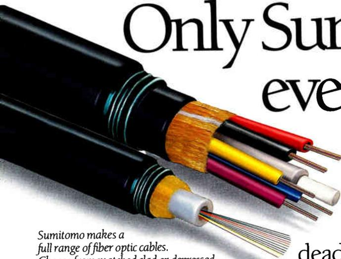
Sumitomo makes a full range of fiber optic cables. Choose from matched clad or depressed clad fiber in either loose tube or LitePipe™ cable construction.
