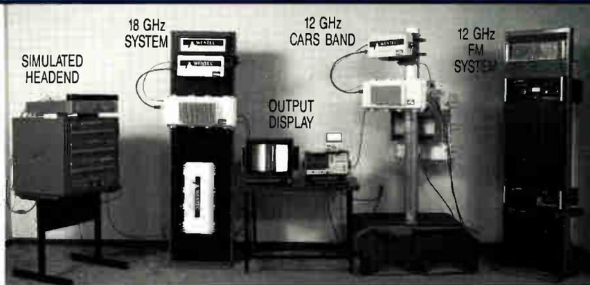
**Microwave Path Simulator Test Facility
