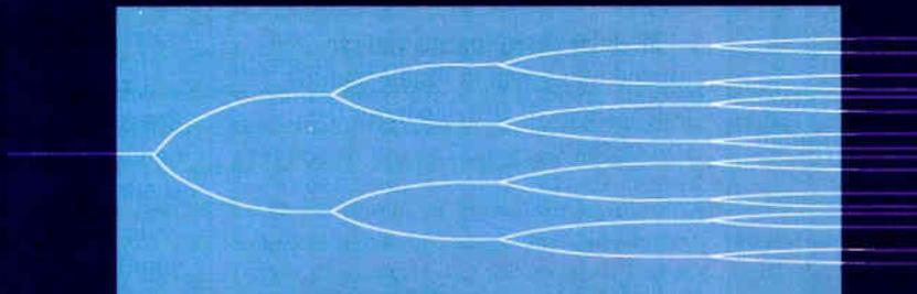
High-port-count planar couplers are produced through passive integration of identical Y-junctions on a small glass chip
