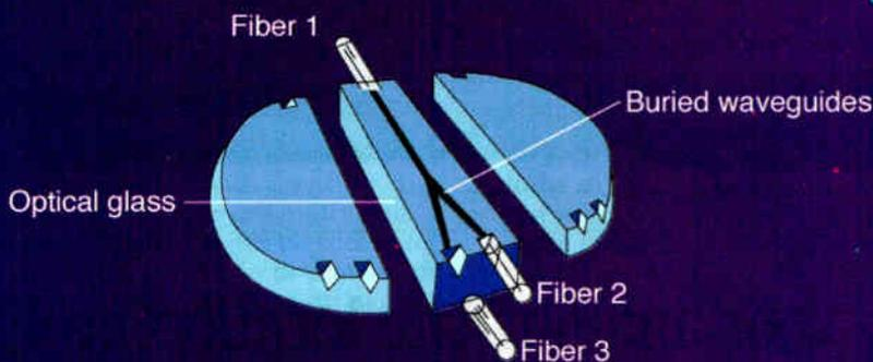
In planar processing, the glass substrate containing optical waveguides is diced, equipped with fiber leads and packaged.
