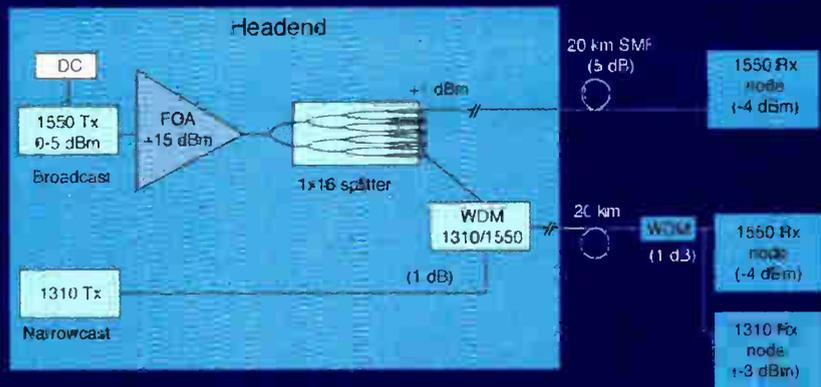
Star cable TV architectures use optical amplifiers and 1x16 splitters to significantly reduce the cost of fiber-optic systems
