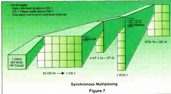
"building blocks," with the basic STS-1 the format that is used throughout the hierarchy. The STS-1 frame consists of: 90 columns of 8-bit bytes, 9 rows of 810 bytes (9 times 90), and 8,000 frames/second. There are a total of 51.84 Mb/s
